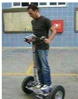
Fig.1 General view of the personal pendulum vehicle
