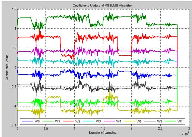
Fig. 5. Noise Channel tracking of the VSSLMS algorithm at SNR -1dB.
