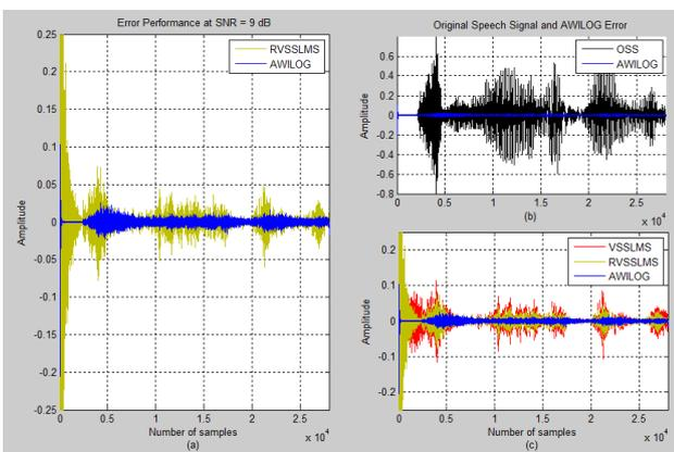
Fig. 12. (a) Shows error between OSS and Cleaned Speech for AWILOG, and RVSSLMS at 9dB SNR, (b) shows OSS and Error of AWILOG, (c) Error between OSS and Cleaned Speech for AWILOG, VSSLMS, and RVSSLMS at 9dB SNR.
