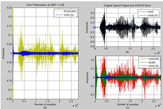
Fig. 15. (a) Shows error between OSS and Cleaned Speech for AWILOG, and RVSSLMS at 3dB SNR, (b) shows OSS and Error of AWILOG, (c) Error between OSS and Cleaned Speech for AWILOG, VSSLMS, and NLMS at 3dB SNR.
