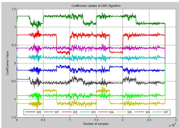
Fig. 6. Noise Channel tracking of the LMS algorithm at SNR -1dB.
