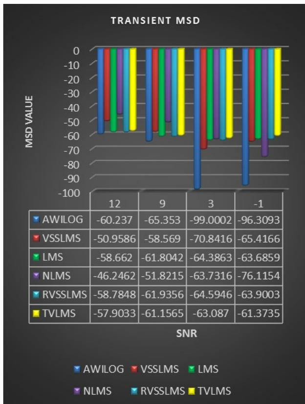
Fig. 3. Transient MSD values versus SNR in the range (12, -1) for various algorithms.
