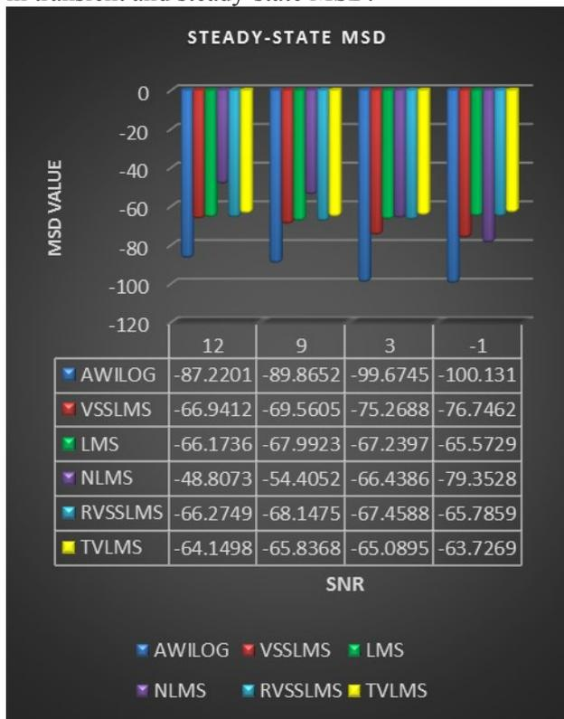
Fig. 2. Steady-state MSD values versus SNR in the range (12, -1) dB for various algorithms.
