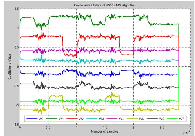
Fig. 8. Noise Channel tracking of the RVSSLMS algorithm at SNR -1dB.
