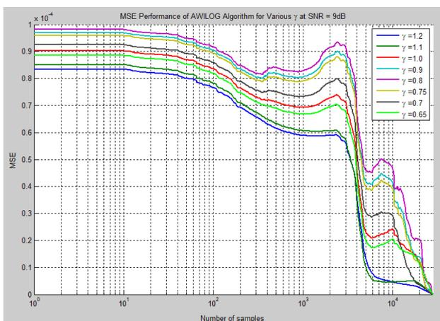
Fig. 20. Shows MSE learning curves of the proposed algorithm for various  $\gamma$  values at 9dB SNR.
