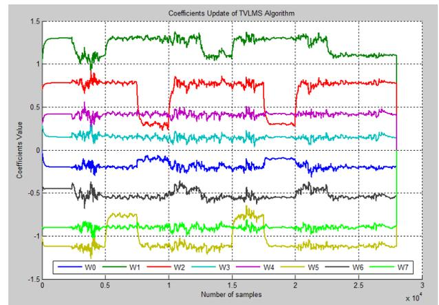
Fig. 9. Noise Channel tracking of the TVLMS algorithm at SNR -1dB.
