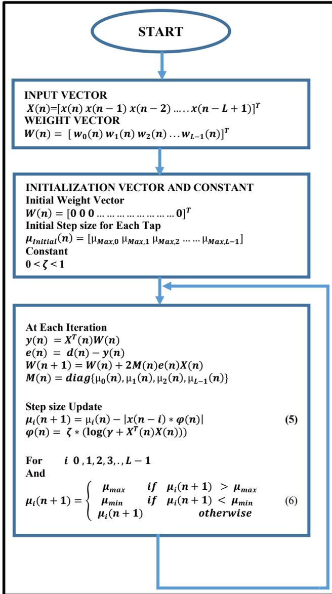
The presence of the parameter  $\gamma$  in the step size adjusting equation is to avoid the restrictive values of the natural logarithmic function. The constant  $\zeta$  is involved to preserve the coefficients adjusting process in the stable area of the adaption process and prevent it to take place in the divergent region. The output accomplishment of the proposed technique delivers an approximately coherent performance for a reasonable range of constant  $\zeta$ . These abilities are
