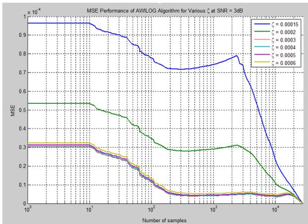
Fig. 19. Shows MSE learning curves of the proposed algorithm for various ( $\zeta$ ) values at 3dB SNR.
