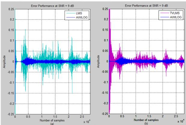
Fig. 11. (a) Shows error between OSS and Cleaned Speech for AWILOG and LMS at 9dB SNR, (b) shows error between OSS and Cleaned Speech for AWILOG and TVLMS at 9dB SNR.
