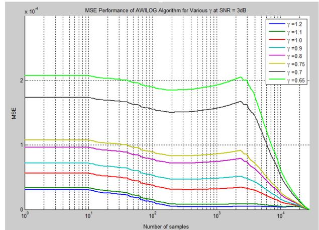
Fig. 21. Shows MSE learning curves of the proposed algorithm for various  $\gamma$  values at 3dB SNR.
