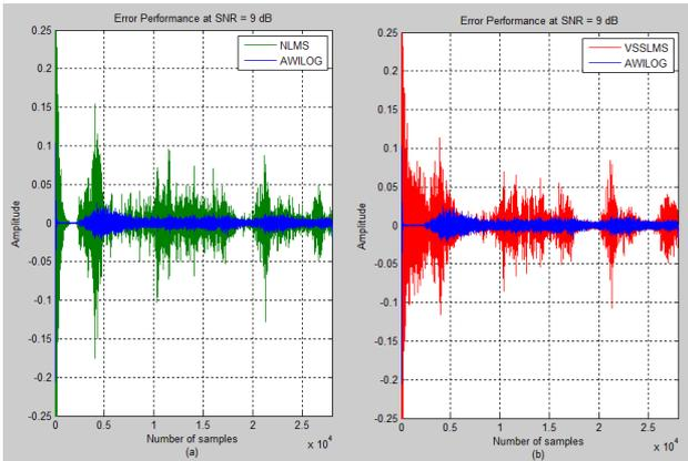
Fig. 10. (a) Shows error between OSS and Cleaned Speech for AWILOG and NLMS at 9dB SNR, (b) shows error between OSS and Cleaned Speech for AWILOG and VSSLMS at 9dB SNR.
