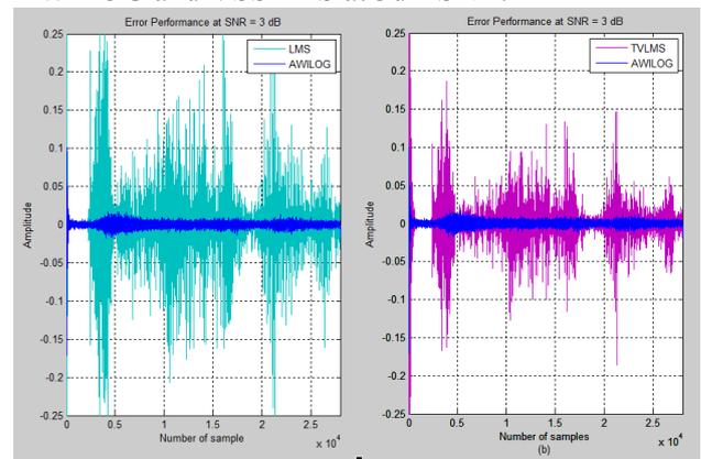
Fig. 14. (a) Shows error between OSS and Cleaned Speech for AWILOG and LMS at 3dB SNR, (b) shows error between OSS and Cleaned Speech for AWILOG and TVLMS at 3dB SNR.
