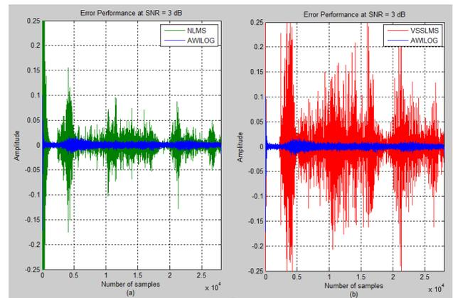
Fig. 13. (a) Shows error between OSS and Cleaned Speech for AWILOG and NLMS at 3dB SNR, (b) shows error between OSS and Cleaned Speech for AWILOG and VSSLMS at 3dB SNR.
