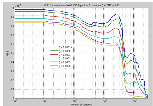
Fig. 18. Shows MSE learning curves of the proposed algorithm for various ( $\zeta$ ) values at 9dB SNR.
