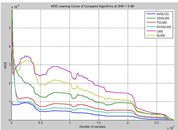
Fig. 16. Shows MSE learning curves of the list of compared algorithms at 9dB SNR.
