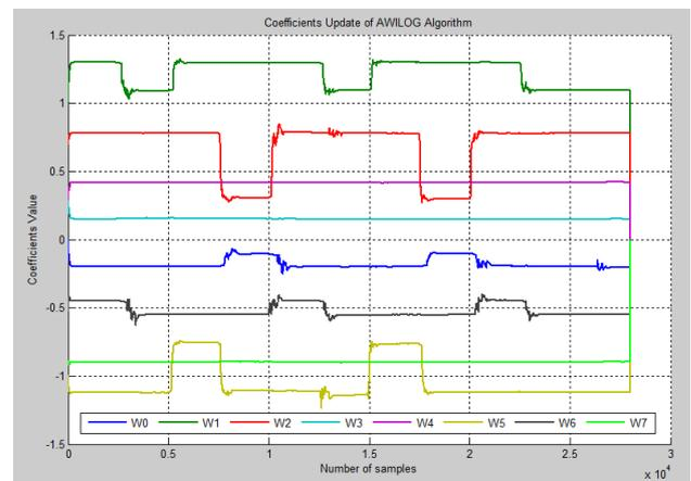
Fig. 4. Noise Channel tracking of the AWILOG algorithm at SNR -1dB.
