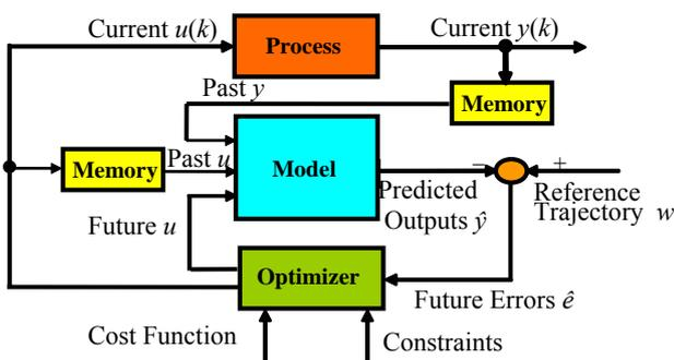
Fig. 4. Block diagram of MPC
