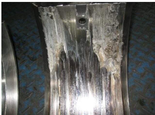
**Fig.18** The maintenance results of the crankpin bearing with fault
