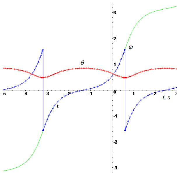
Fig.6 The numerical integration (lines) and analytical (points) results for the Euler angles
