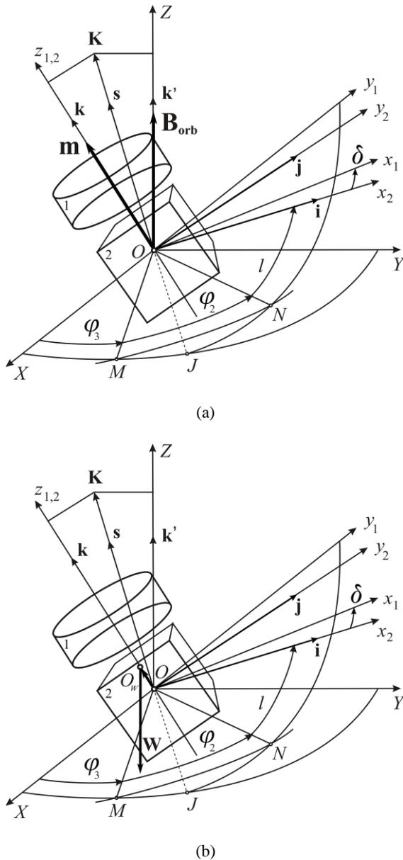
Fig.2 The magnetic DSSC coordinate frames (a) and the "heavy coaxial top" (b) with the Andoyer-Deprit coordinates
