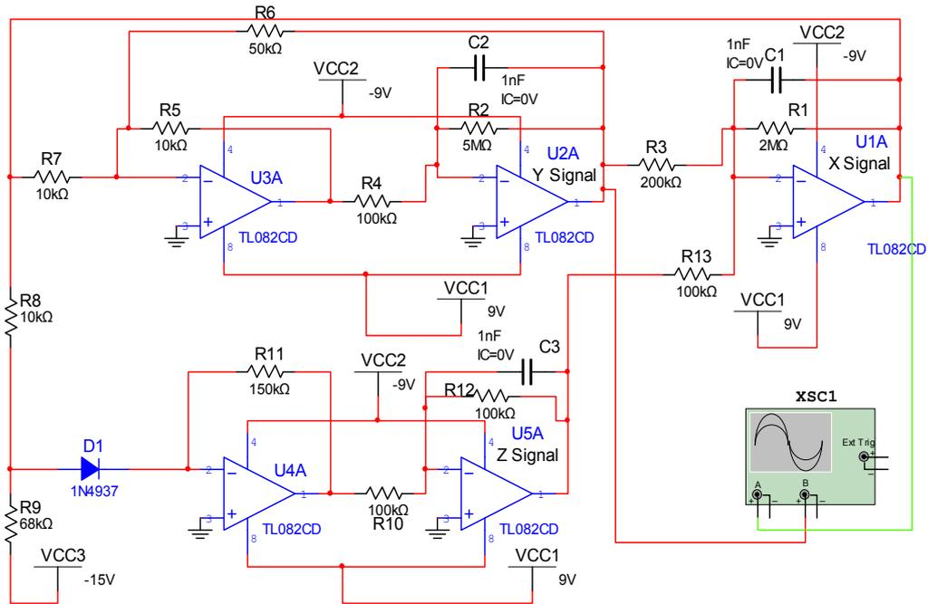
Fig. 3. Schematic of the proposed Rossler circuit
