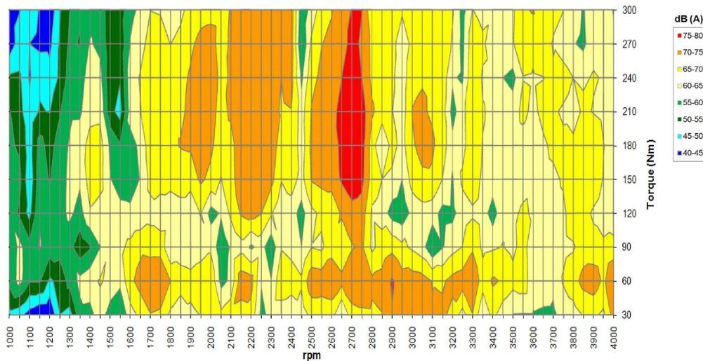
Fig. 10 - ColorMap - Microphone - Order of meshing gear - 4<sup>th</sup> gear, maker A
