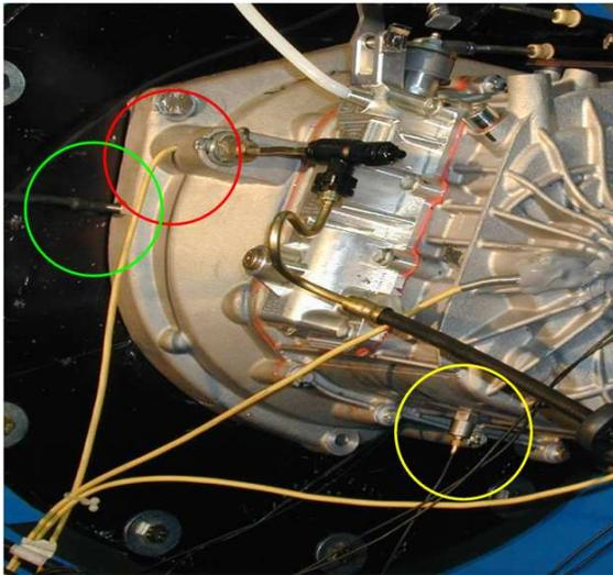
Fig. 9 – The set-up of the gearbox: the accelerometer (yellow), the pick-up (green) and the thermocouple (red)
