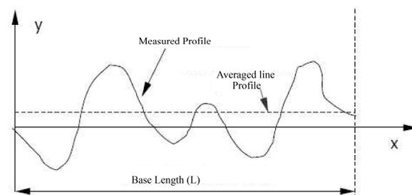
Fig. 3 – The determination of the average line reference
