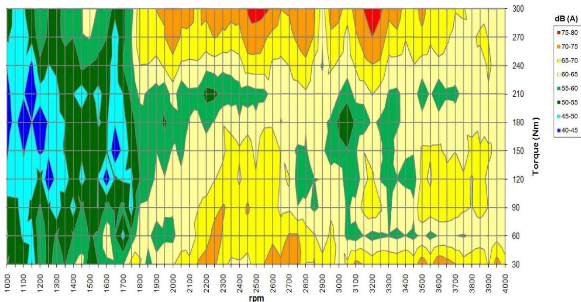
Fig.16 - ColorMap - Microphone - Order of meshing gear - 4<sup>th</sup> gear, gear-box A modified
