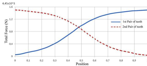
Fig. 6 – Distribution of forces between two pairs of meshing teeth
