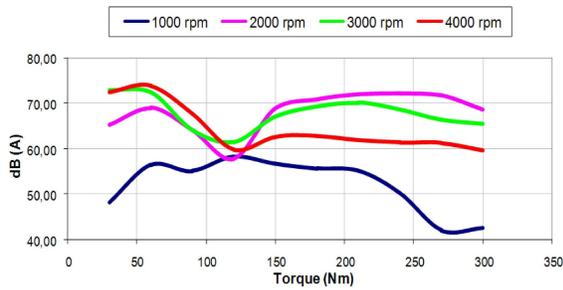
Fig.12 – Acoustical pressure vs applied torque, in 4<sup>th</sup> gear, for several rpm
