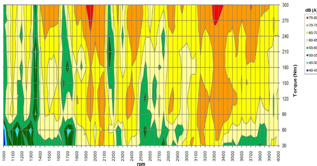
Fig.11 - ColorMap - Microphone - Order of meshing gear - 4<sup>th</sup> gear, maker B
