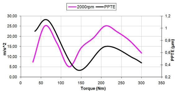
Fig.14 – Comparison of vibration and PPTE vs applied torque, in 4<sup>th</sup> gear, at 2000rpm
