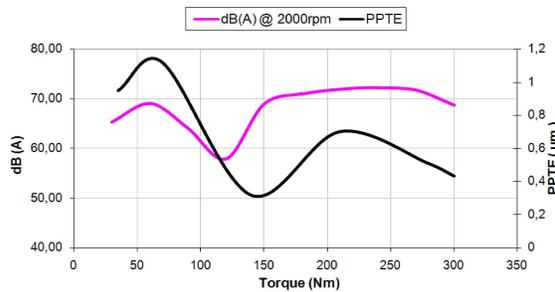
Fig.13 – Comparison of acoustical pressure and PPTE vs applied torque, in 4<sup>th</sup> gear, at 2000rpm
