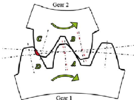
Fig. 1 - Meshing gear: red colour highlights the early contact
