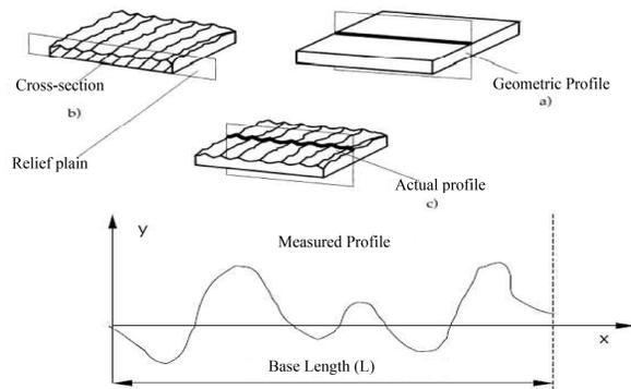
Fig. 2 – The definition of the roughness
