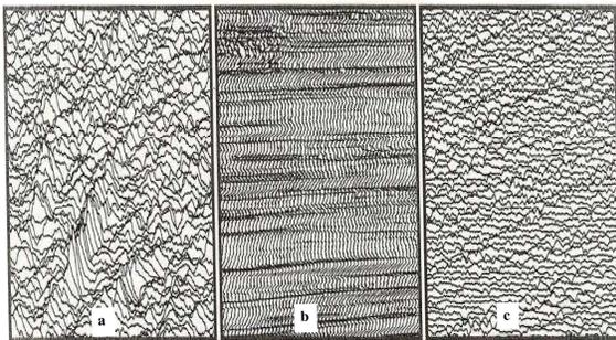
Fig. 4 – The texture of surface generated by three different finishing methods
