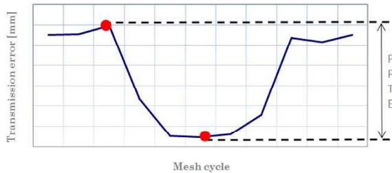
Fig. 5 - Peak to Peak Transmission Error
