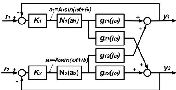
Fig.2. A 2x2 Nonlinear Multivariable Feedback Control System.
