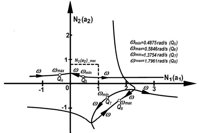
Fig.8. Root-loci Analyses of limit cycles of Example 1 for  $k_1 = k_2 = 1$ .
