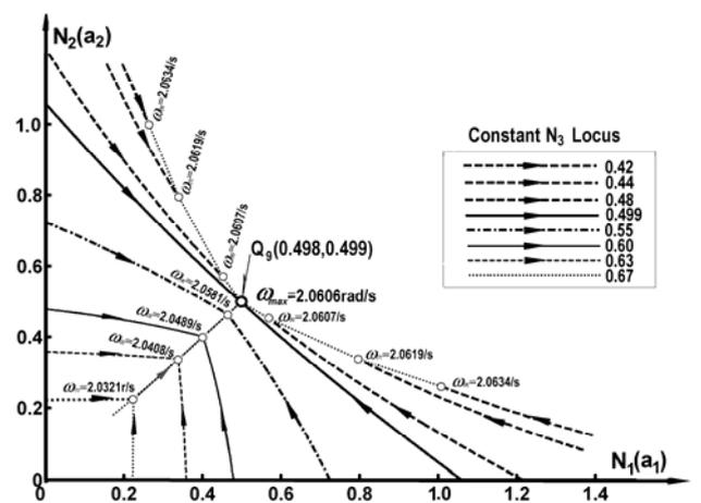
Fig.10. Root-loci analyses of limit cycles of Example 2 on  $N_1(a_1)$  vs.  $N_2(a_2)$  Plane for  $N_3(a_3)$  varying and  $k_i = 1$ .
