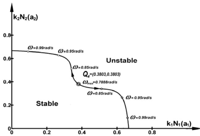
Fig.6. Root-Loci of limit cycles in the parameter plane.
