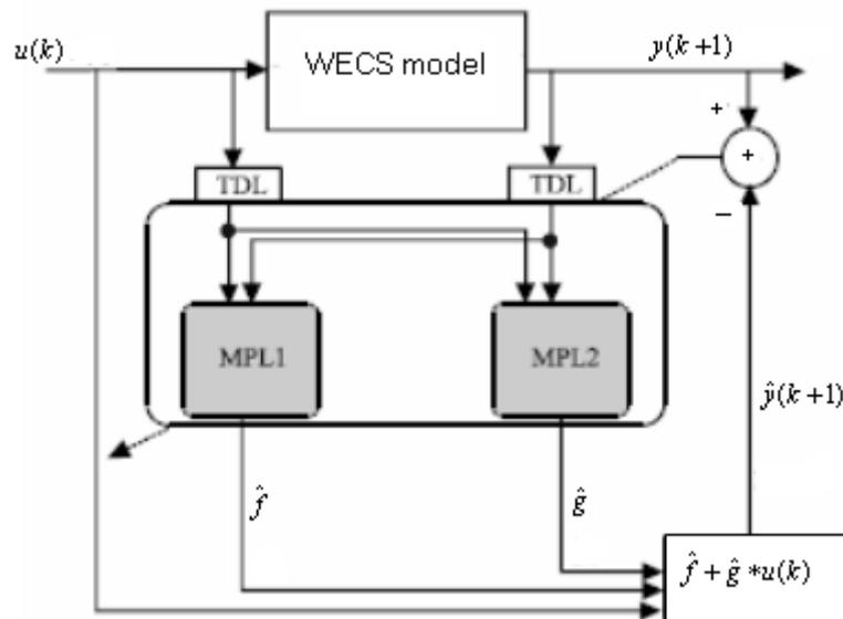
Fig. 2: NARMA-L2 plant model identification
