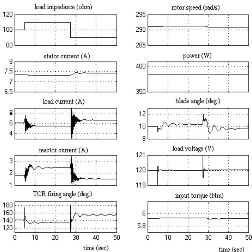
Fig. (6): Dynamic response of proposed system with step change in load impedance.
