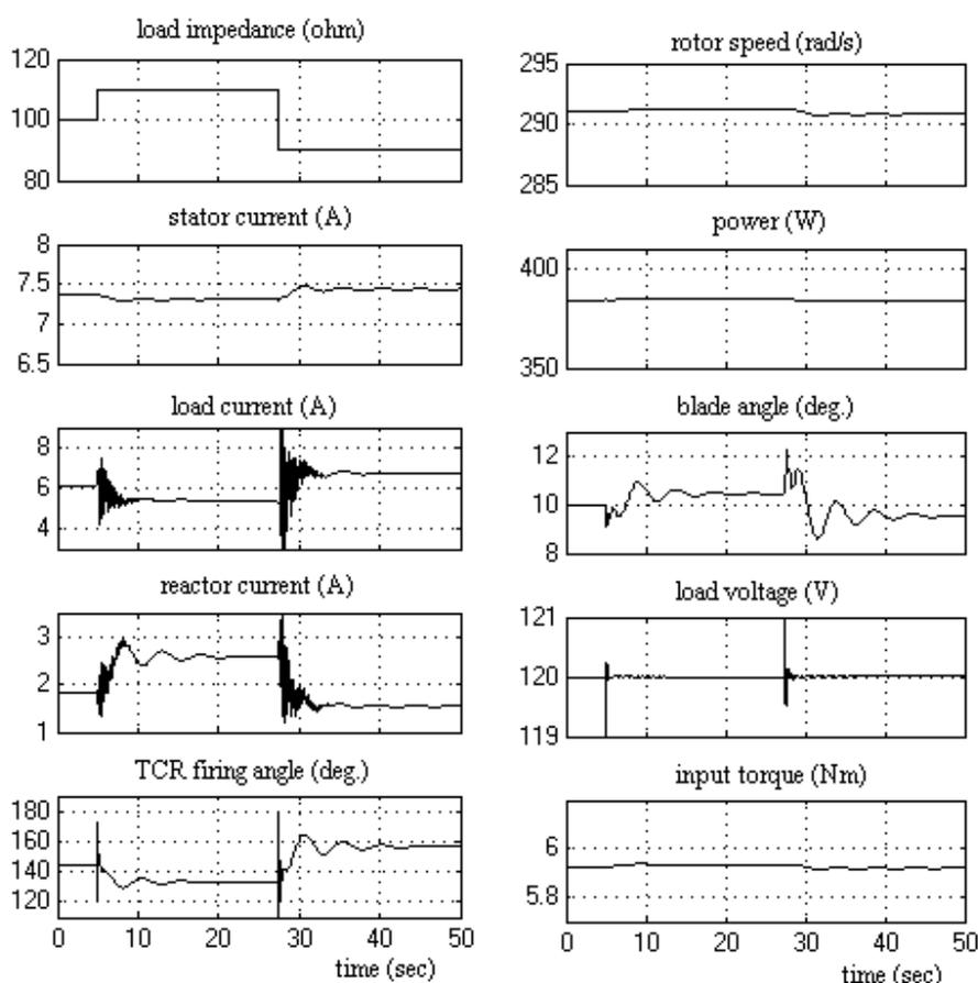
Fig. (8): Dynamic response of the proposed system with a step change in load impedance and parameters changes.
