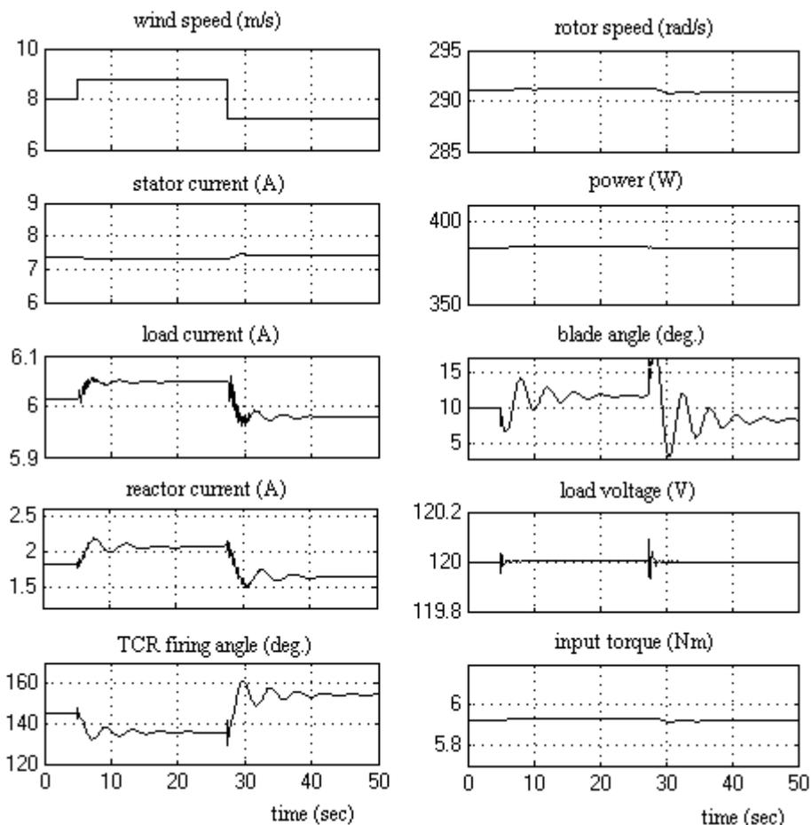
Fig. (5): Dynamic response of proposed system with step change in wind speed.
