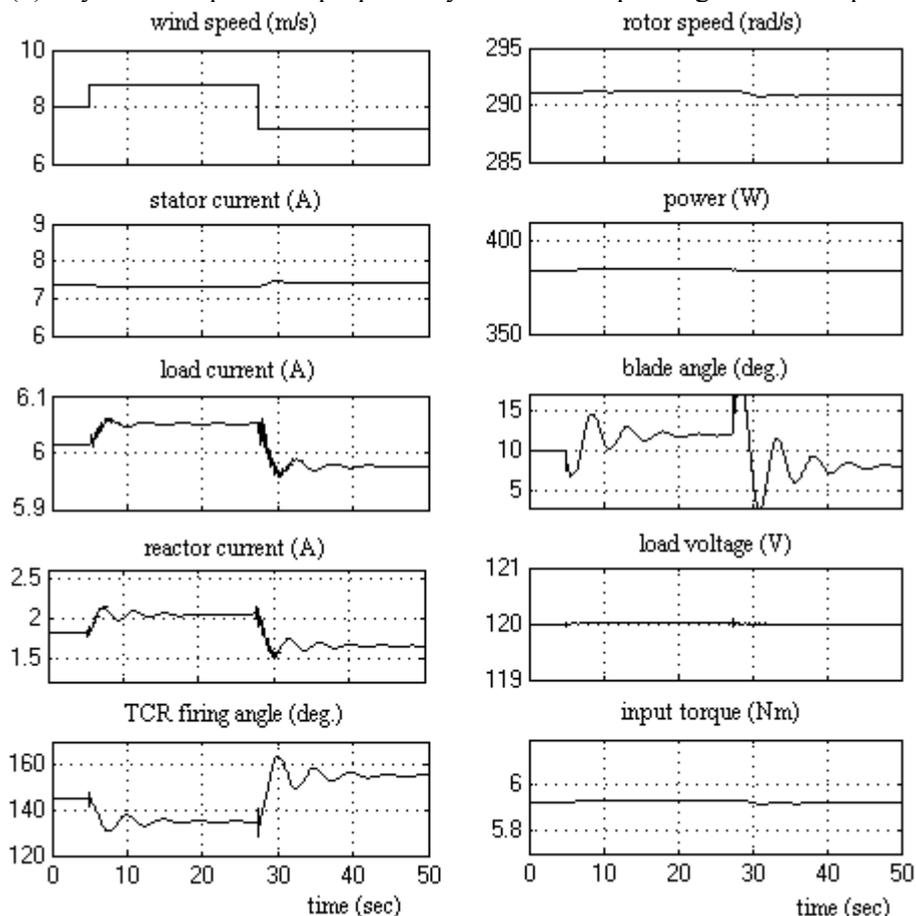
Fig. (7): Dynamic response of the proposed system with a step change in wind speed and parameters changes.
