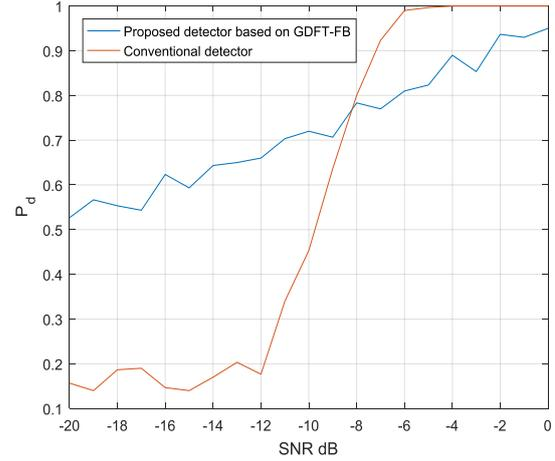
Figure 1: Performance comparison between the proposed detector and Conventional detector for 8-PSK
