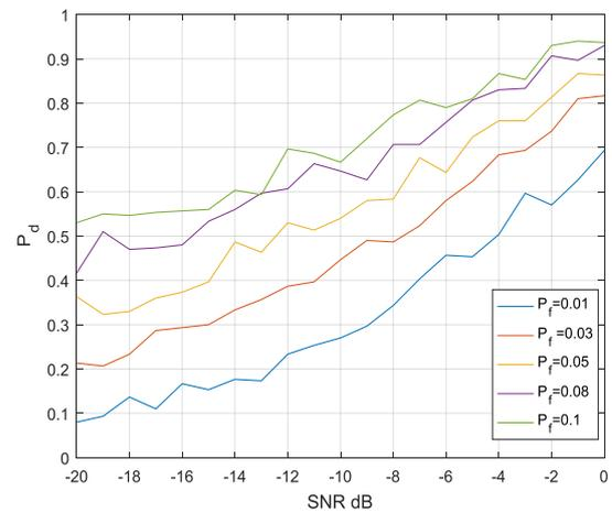
Figure 2: ROC of the proposed detector and Conventional detector for 8-PSK
