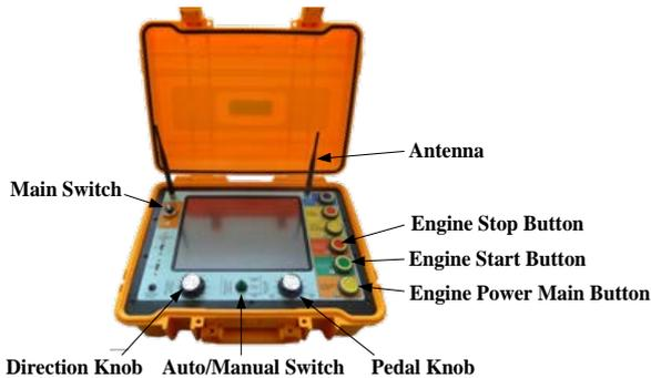
Fig. 8 The shore-based controller
