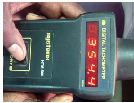
Figure.20.Motor speed in BLDC hub motor
