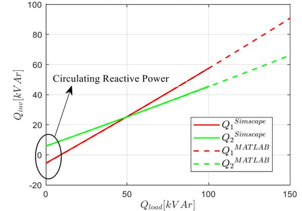
Fig. 10: Comparison between simplified solution and Simscape simulation:  $Q_{10} = 25$  kVAr.
