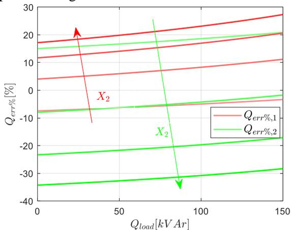
Fig. 5: Reactive power sharing errors with variable connection impedance.
