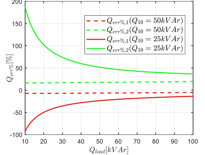
Fig. 9: Reactive power sharing errors.
