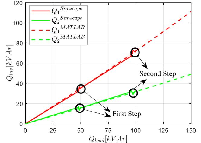
Fig. 7: Comparison between simplified and detailed simulation for reactive power sharing.
