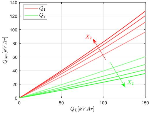
Fig. 3: Reactive powers as a function of  $X_1$  and  $X_2$ .
