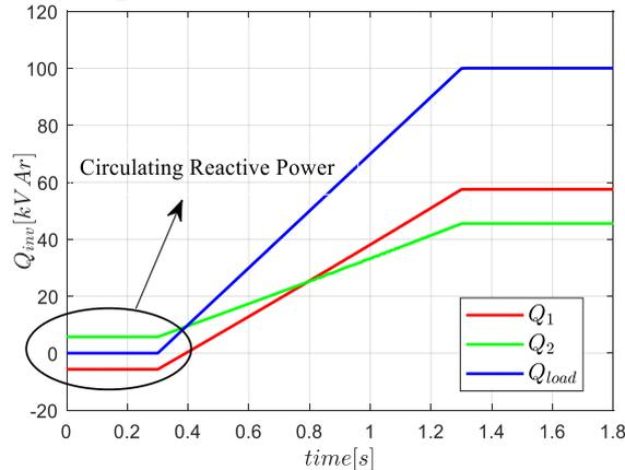
Fig. 8: Reactive power time profile:  $Q_{10} = 25$  kVAr.
