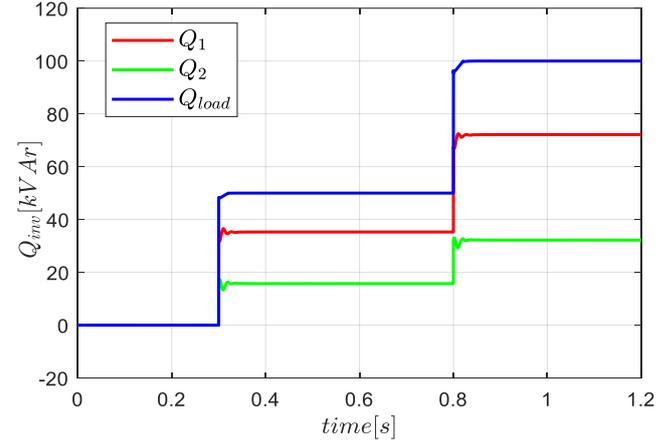
Fig. 6: Reactive power time profiles.
