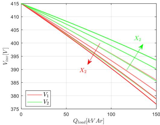
Fig. 4: Voltages as a function of  $X_1$  and  $X_2$ .
