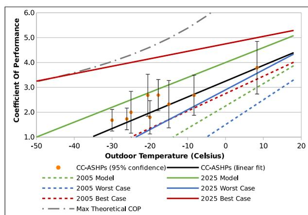
Figure 4: Technological development of heat pump performance.
