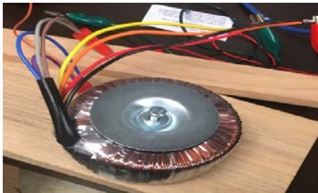
Fig. 13 Toroidal Transformer used
