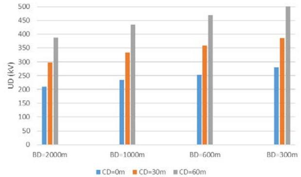
**Fig. 5** The developed overvoltages at position D ( $U_D$ ) in function with the distance CD and the cable length BD in case of a lightning hit on the phase conductor of the connected transmission line
