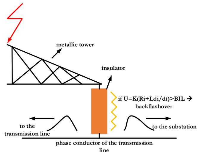
**Fig. 6** Lightning hit on the metallic tower of an overhead transmission line
