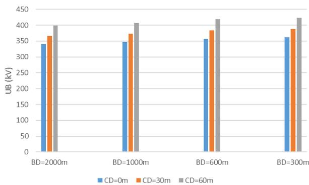
**Fig. 4** The developed overvoltage at position B ( $U_B$ ) in function with the distance CD and the cable length BD in case of a lightning hit on the phase conductor of the connected transmission line
