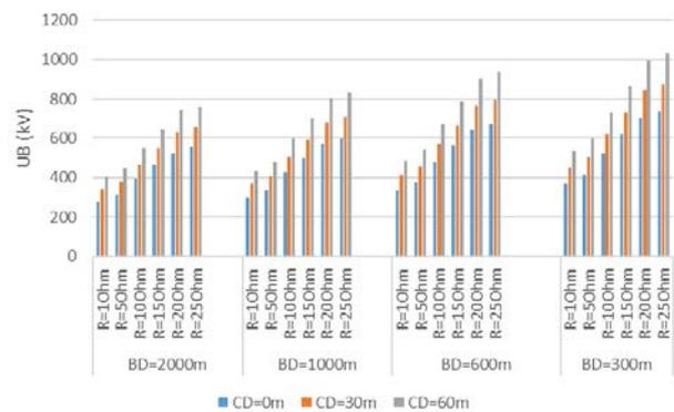
**Fig. 9** The developed overvoltages at position B ( $U_B$ ) in function with the installation position of the arresters CD, the tower footing resistance ( $R$ ) and the cable length BD in case of a lightning hit on the ground wire of the connected transmission line
