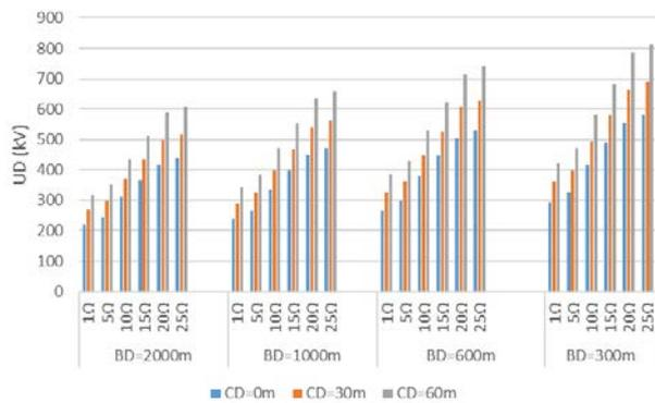
**Fig. 10** The developed overvoltages at position D ( $U_D$ ) in function with the installation position of the arresters CD, the tower footing resistance ( $R$ ) and the cable length BD in case of a lightning hit on the ground wire of the connected transmission line
