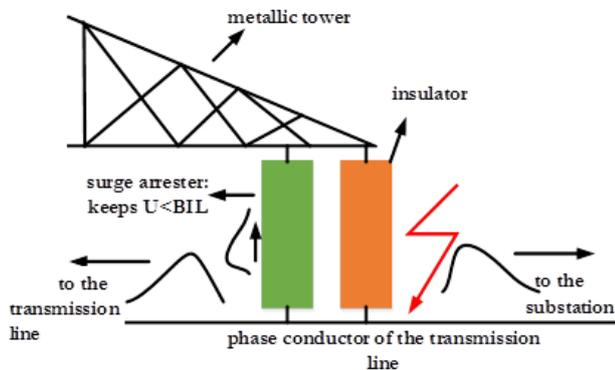
**Fig. 7** Overhead transmission line protected by surge arresters
