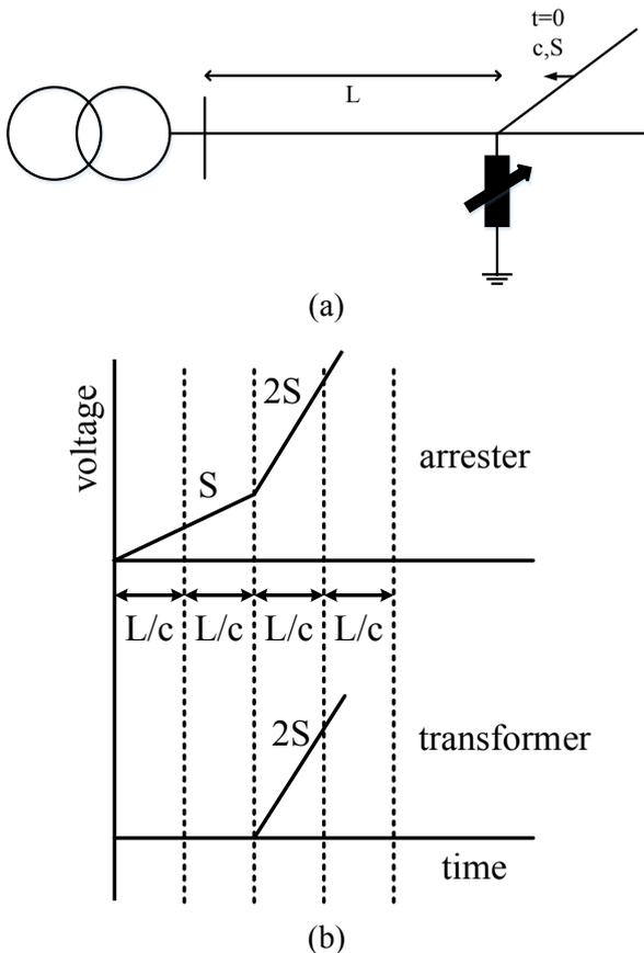
**Fig. 1** (a) Power transformer protected by a surge arrester, (b) Developed overvoltages at the terminals of the arrester and the transformer ( $S$  is the steepness of the lightning surge,  $c$  is the light velocity,  $L$  is the distance between the transformer and the arrester)
