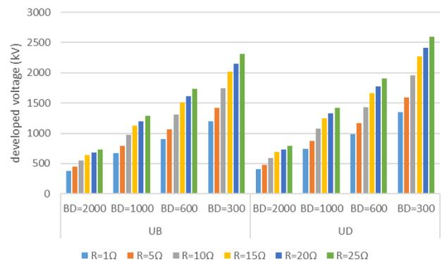
**Fig. 8** The developed overvoltages at position B ( $U_B$ ) and D ( $U_D$ ) in function with the length of the cable BD and the tower footing resistance ( $R$ ) (no arresters) in case of a lightning hit on the ground wire of the connected transmission line
