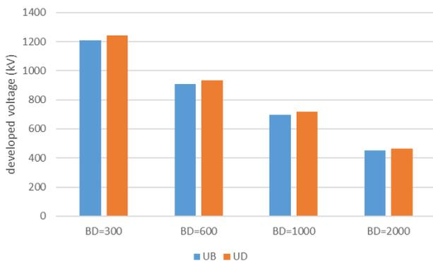
**Fig. 3** The developed overvoltages at positions B ( $U_B$ ) and D ( $U_D$ ) in function with the length of the cable BD in case of lightning hit on phase conductor of the connected line (no arresters)
