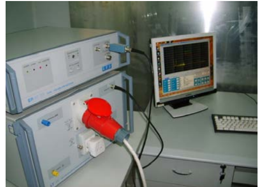
Fig.24 Test system of CM conducted interference
