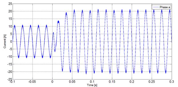
Fig.8 AC Current - case 2 (phase a)
