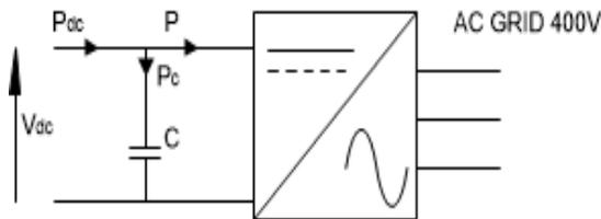
Fig.3 Power exchanges on DC link
