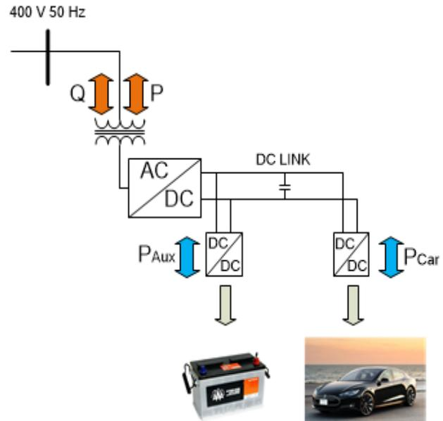
Fig.1 Technical scheme of the charging station
