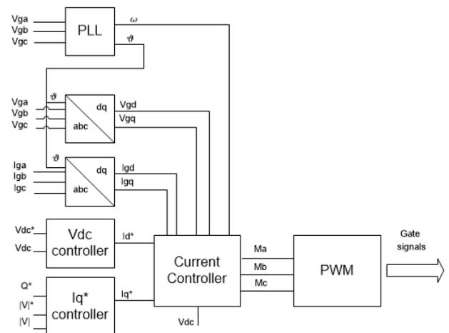
Fig.2 AC/DC converter control scheme
