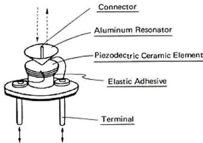
Fig 2: Topology of Ceramic-Film Ultrasonic Transducer
