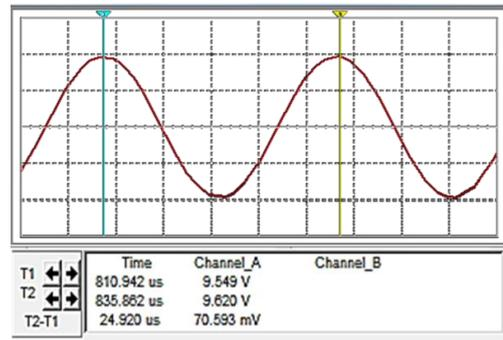
Fig. 6. Output waveform of push-pull converter simulation result
