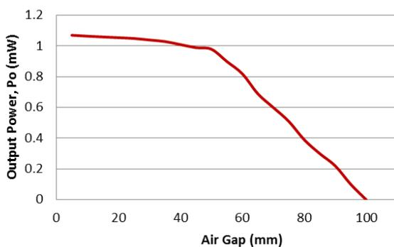
Fig.13: AET system with different air gap between transducers
