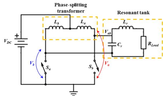
Fig. 3. Basic circuit of push-pull converter.
