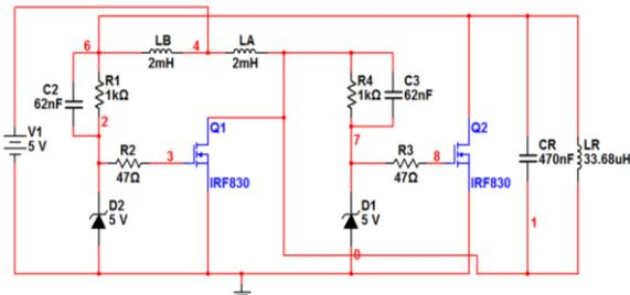
Fig. 5 : Push-pull power converter schematic circuit
