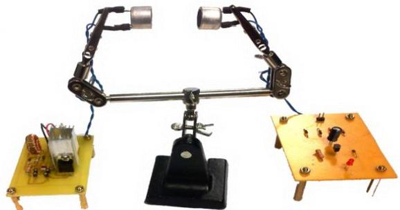
Fig. 9: AET basic system using push-pull power converter transmits energy through the air medium.
