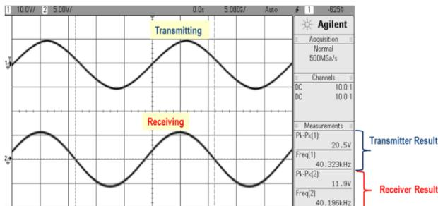
Fig. 7: Result of transmitting voltage from function generator
