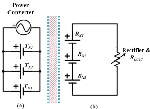
Fig.16: (a) Connection of multiple transmitters, Tx in parallel (b) Connection of multiple receivers, Rx in series
