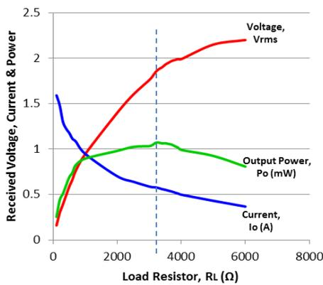
Fig. 12: The optimal power transfer ratio obtained by the varying the load resistance value. The most optimum value is at 3.3kΩ load resistances where 1.071mW power.
