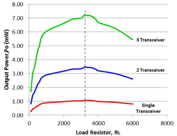
Fig.17: Result of multiple input-output AET system. The maximum power of the system is 1.07mW for single transceiver, 3.47mW for 2 transceivers and 7.24mW power for 3 transceivers.
