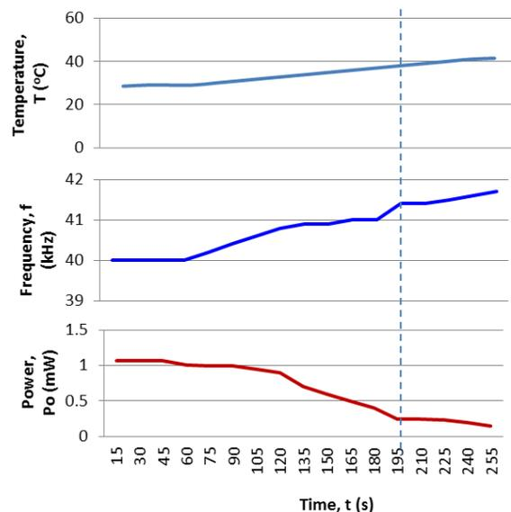
Fig. 14: The effect of capacitor's temperature to the frequency and the transferred power.
