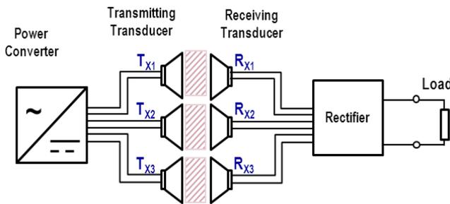
Fig.15: Multiple input-output AET system block diagram
