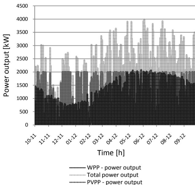
Fig. 4 One year data of output power from the hybrid system for Case I - hourly values
