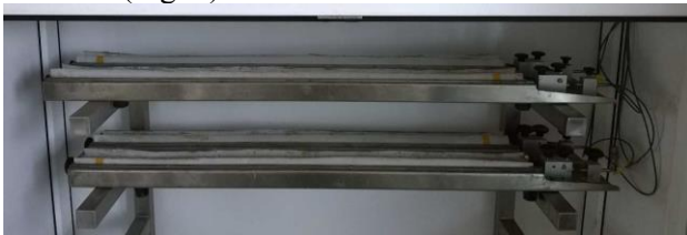
Fig. 2 – Shrinkage-drains in air-conditioned chamber
