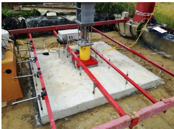
Fig.1 Typical concrete slab with dimensions 2 x 2 m during testing
