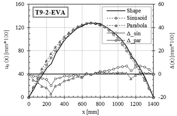
Fig. 7 Typical and untypical specimen: Shapes of imperfection and their approximation
