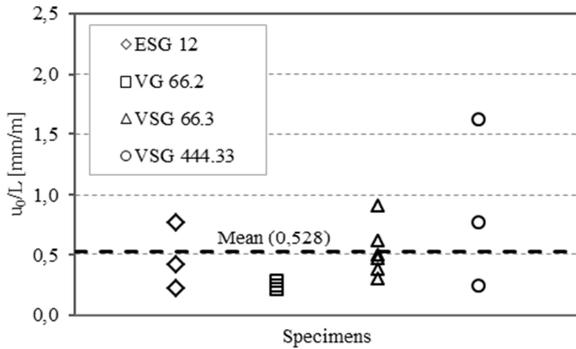
Fig. 6 Amplitudes of initial imperfections of tested specimens
