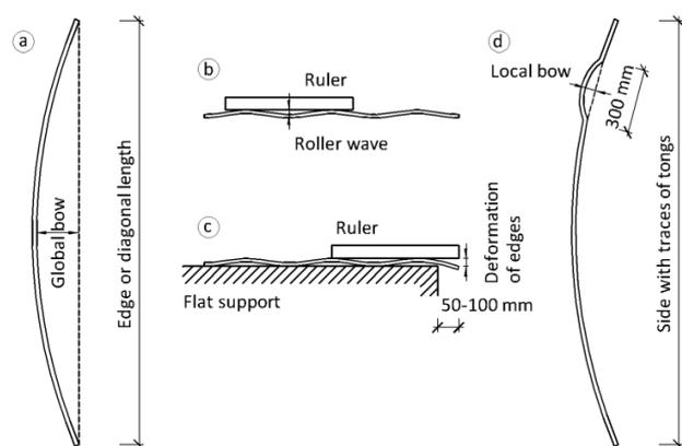
Fig. 2 Glass pane deformations types
