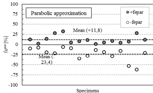
Fig. 8 Fitting errors and mean values; approximation by sinusoid and parabola
