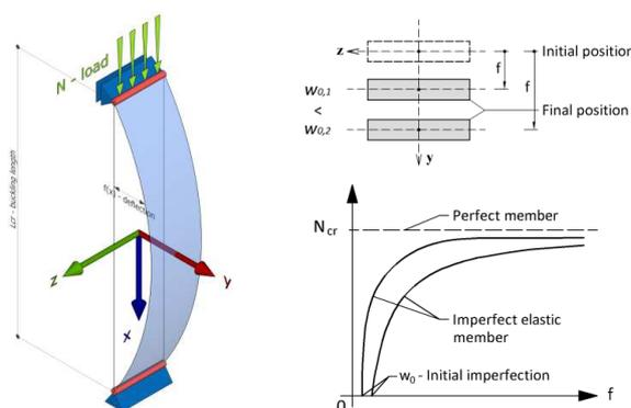
Fig. 1. Flexural buckling of slender beam, load-deflection curve of perfect and imperfect member
