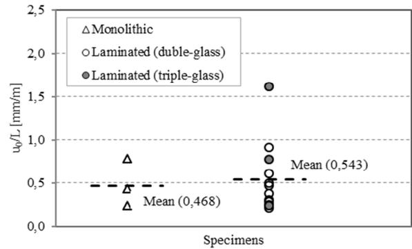
Fig. 9 Influences on imperfections; glass type effect (upper); lamination effect (bottom)
