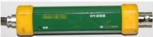
Fig.17 Signal conditioner/amplifier
