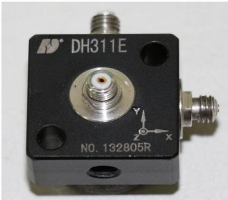
Fig.15 IEPE three directions piezoelectric acceleration sensor
