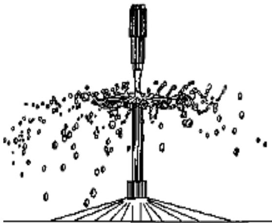
Fig. 8 Vibration jet decay
