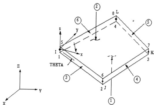
**Fig.(5):Shell 63 used in building the foundation models**
