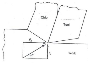
**Fig.(2): Thrust and Tangential and their resultant**
