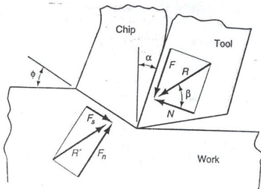
**Fig.(1):Cutting force components**
