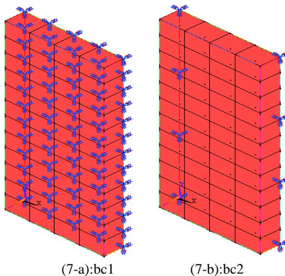
**Fig.(7): Types of boundary conditions.**
