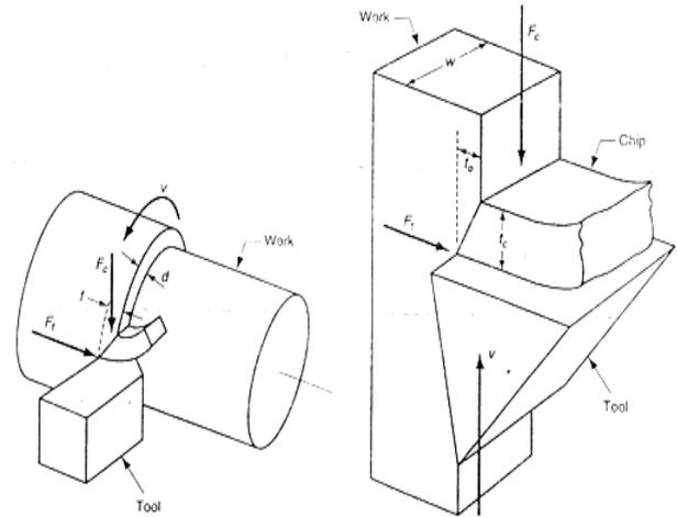
**Fig.(4): Orthogonal cutting force components**
