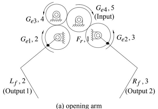
Figure 9 Schematic diagram of a new (5,7) robot arm
