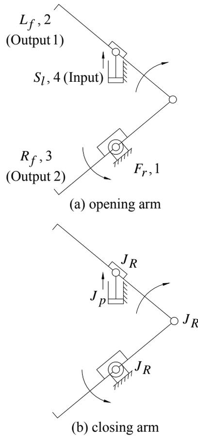
Figure 6 Schematic diagram of another (4,4) robot arm
