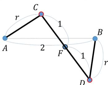
Figure 2 is a description of a three-bar linkage system:  $A$  and  $B$  are fixed points;  $AC$ ,  $CD$ ,  $DB$  are rods;  $C$  and  $D$  are hinge points;  $AC$  is the driver and  $C$  is the mover rotating around the fixed point  $A$ ;  $F$  is the marker.
