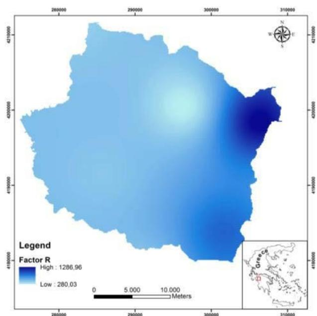
**Fig.4:** Rainfall-Runoff Erosivity Factor (R) map of the basin of Pineios dam
