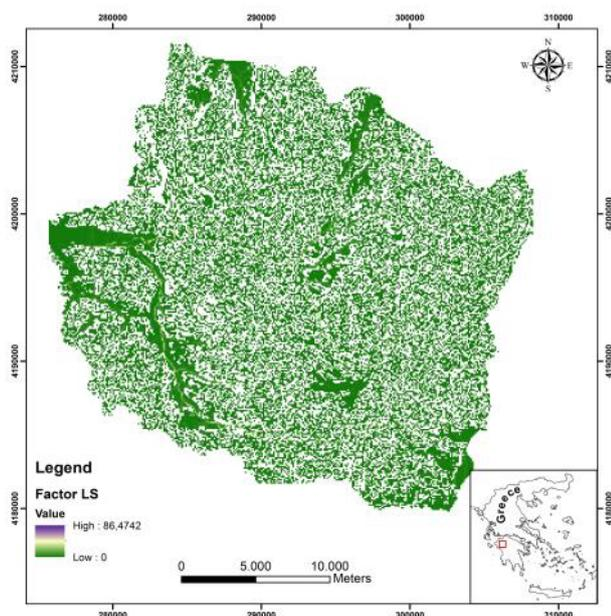
**Fig.6:** Slope length and steepness factor (LS) map of the basin of Pineios dam
