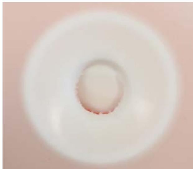
Fig. 11. PP deformation after drop weight test at 100 J.
