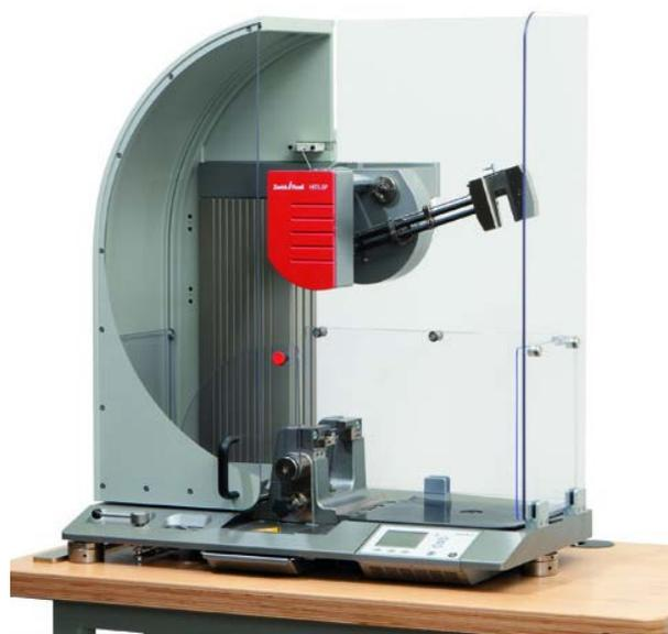
Fig. 6 Impact bending test
