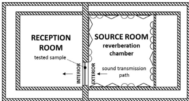
Fig. 3. Schematic of laboratory layout and location of the tested sample.
