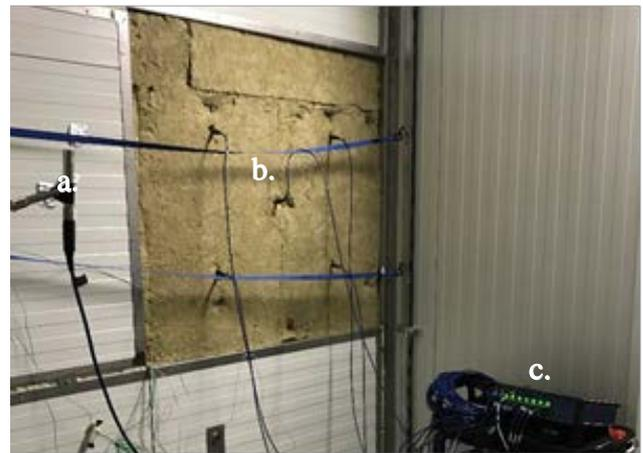
Fig. 5. Measurement of the standardized level difference in the Laboratory (a.  $L_{pA}$  measurement in reception room, b. Microphone field, c. Norsonic MF-850).
