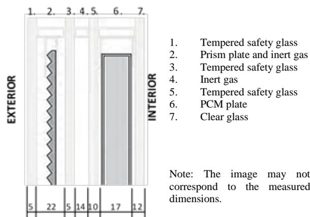
Fig. 1. Description of layers of quadruple glazing panel.
