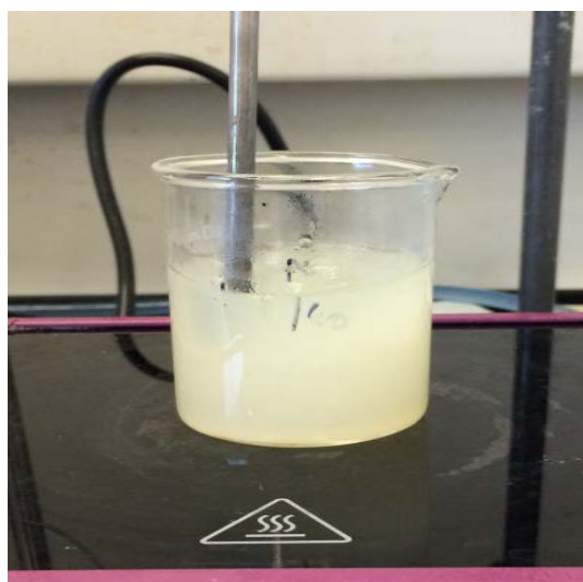
Figure 3: PE precipitation during cooling after dissolution
