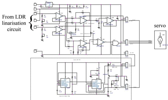
Figure 19: Feedback loop Control circuit
