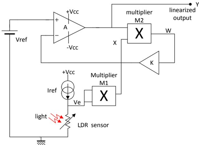
Figure 9: Full circuit diagram
