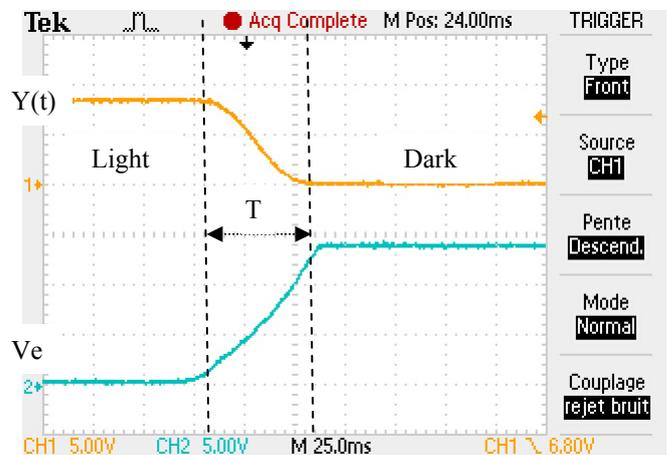
Figure 18: transient response to a step of luminous flux
