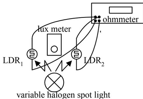
Figure 3: LDR test bench
