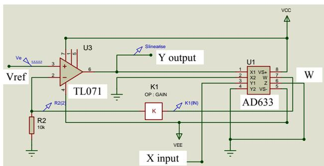
Figure 6: Hyperbolic circuit schematic
