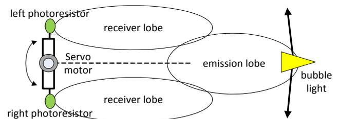
Figure 2: Bubble light alignment
