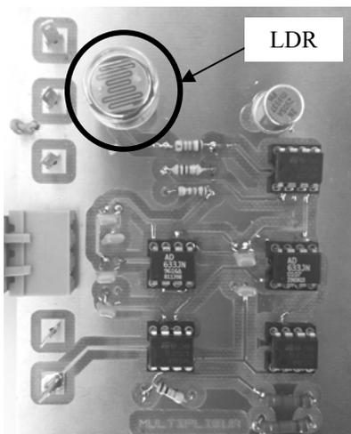
Figure 16: LDR test circuit
