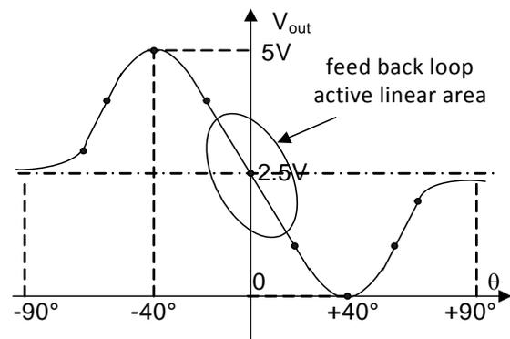
Figure 22: LDR’s  $V_{out}$  voltage difference vs. light axis angle  $\theta$  (in degrees)
