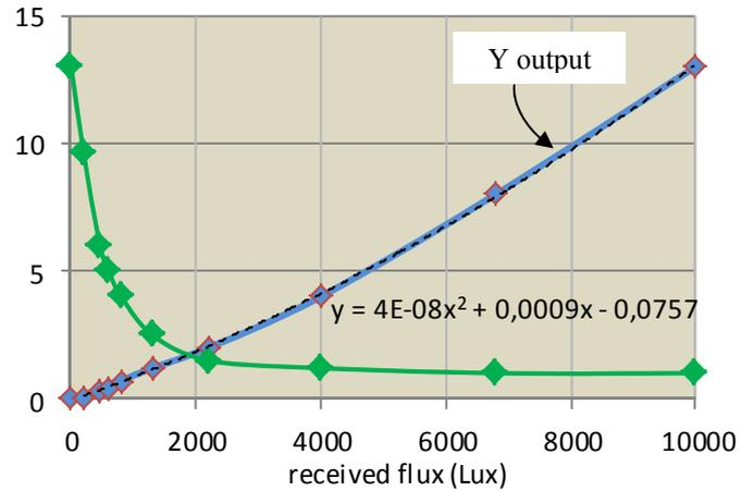
Figure 17: experimental linearization curve
