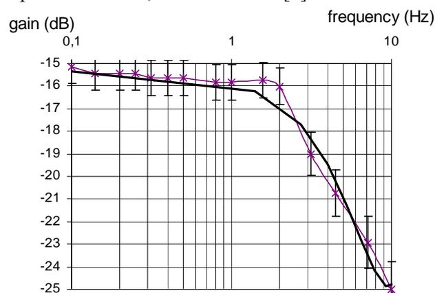
Figure 24: Experimental AC open loop gain  $V_{out}/V_{in}$
