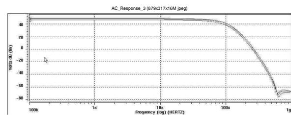
**Figure 11.** AC Response of four corner simulation in HSPICE
