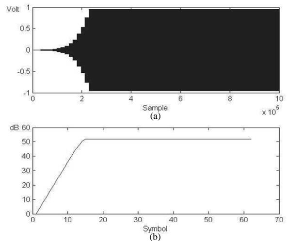
**Figure 10.** AGC close-loop simulation with settling time using Matlab
