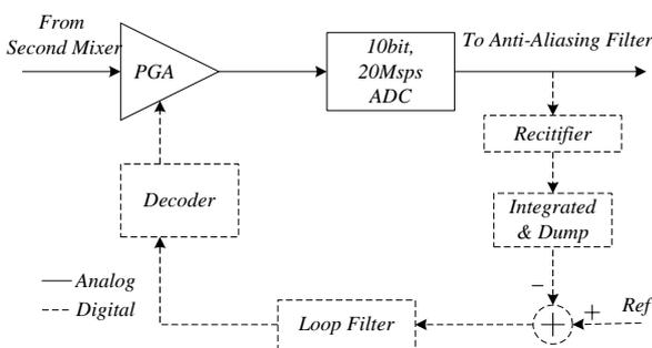
Figure 2. Block diagram of the proposed AGC
