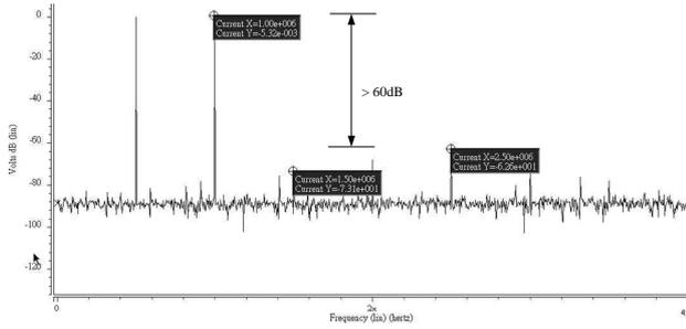
**Figure 8.** Simulation PGA's output two-tone spectrum at 1 Mhz; 500 kHz and 80  $mV_{pp}$  output. The third order intermodulation is less the 60 dB.
