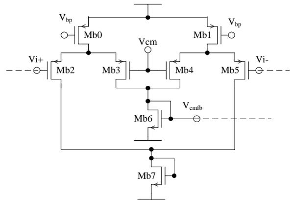
Figure 7. Common mode feedback circuitry
