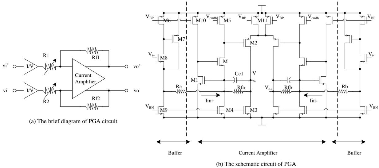
Figure 4. The Programmable-Gain Amplifier circuit
