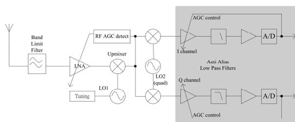
**Figure 1.** A typical architecture of wideband IF receiver with double conversion.
