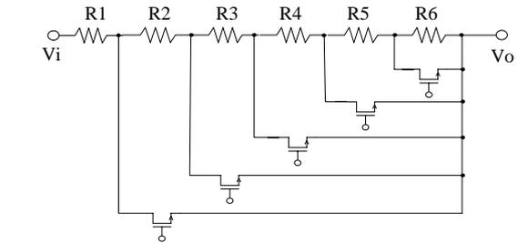
Figure 6. Schematic of Variable Input Resistors
