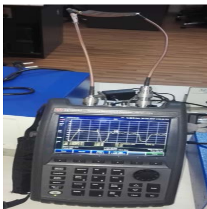
Fig.9 Experimental setup for testing the filter
