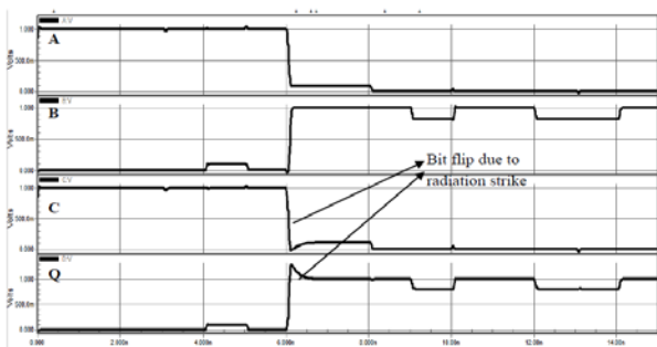
Fig. 15 SEDU output of Modified TDICE D flip flop at node QR and C
