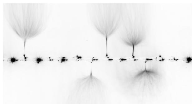
Fig. 3 Example of reflective method (inversed image) using collimated light - with good visibility flexural instability, but with significant spot reflections on drops on the spinning electrode (wire). Contour and shape of liquid are difficult to see.
