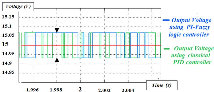
Fig.10 Output voltage ripple.
