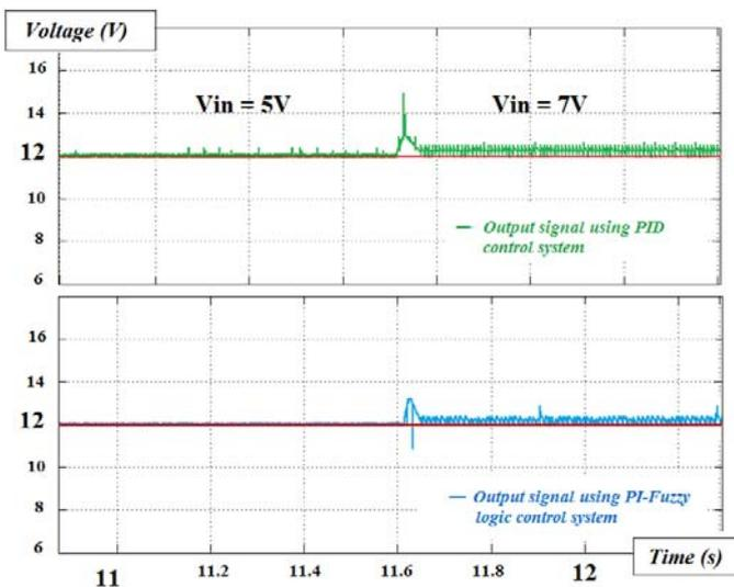
Fig.7 Simulation with irregular supply voltage.
