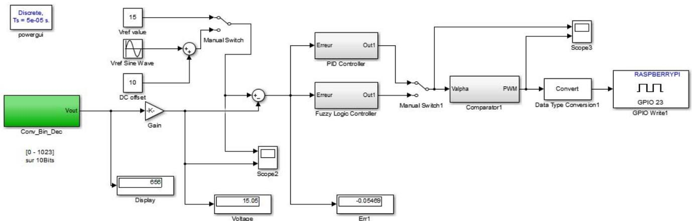
Fig.4 Block diagram of the implemented control system.
