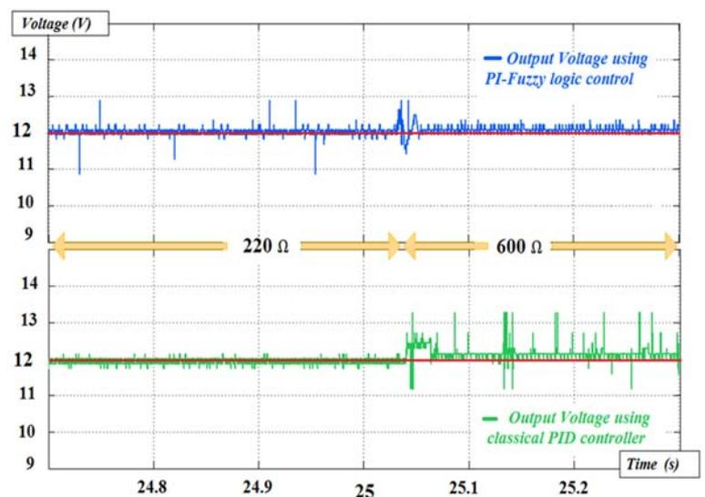
Fig.8 Output voltage for load change case.
