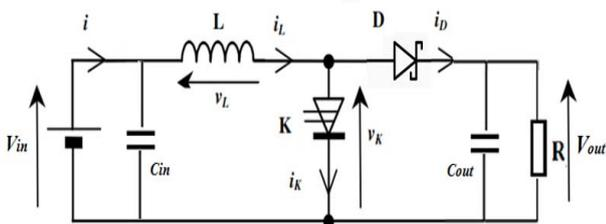
Fig.2 Topology of the Boost converter.
