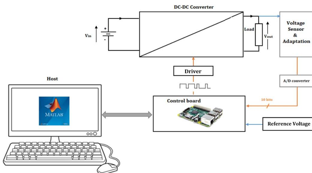
Fig.1 The proposed block diagram system.
