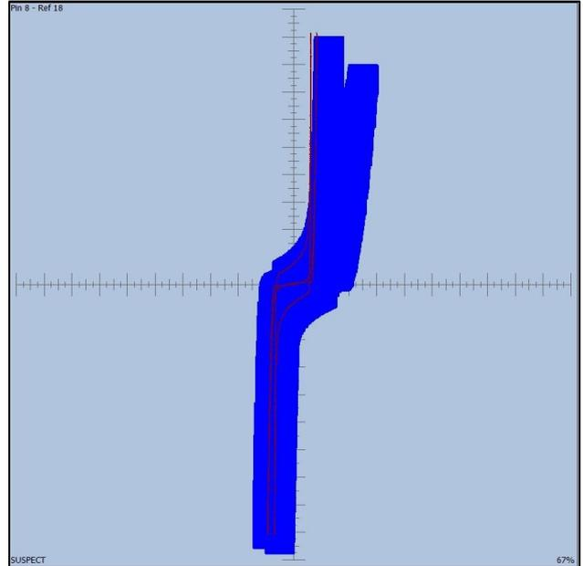
Fig. 9 Dual pin print affected by laser ablation process.
