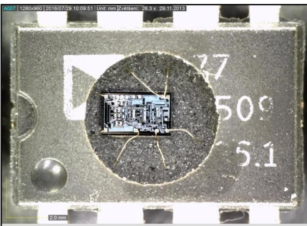
Fig. 61 OP177 by AD package marking in direct vertical lighting combined with radial lighting.
