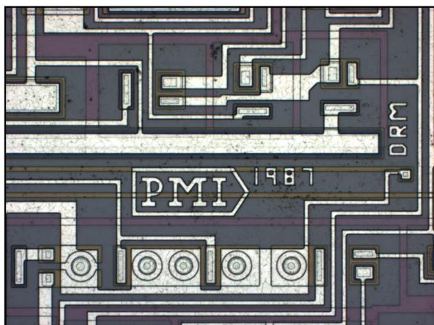
Fig. 65 Revealed PMI chip logo and date with polarization microscope magnification set to 200.
