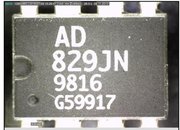
Fig. 26 Radial white colour lighting in combination with direct vertical white lighting.
