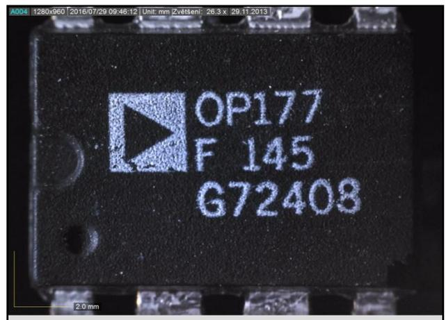
Fig. 58 OP177 component by alleged AD package labeling illuminated with oblique lighting.
