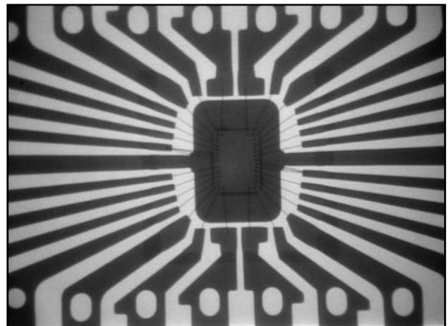
Fig. 31 Same type of EEPROM with distinct contact terminal system X-ray image.
