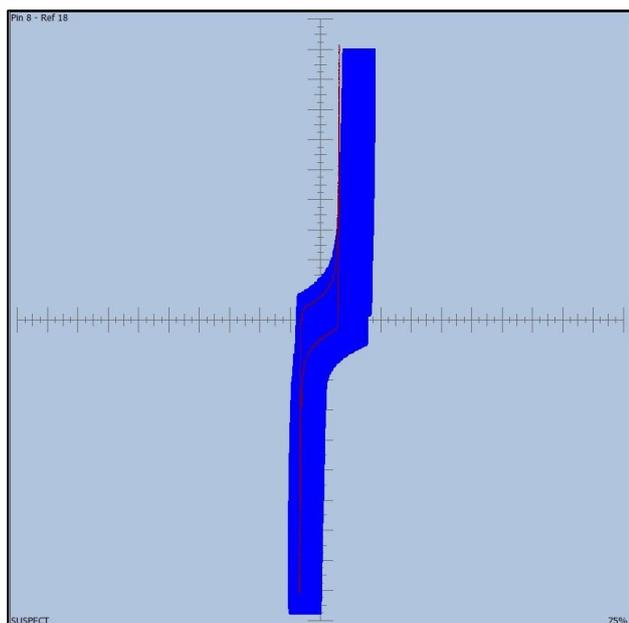
Fig. 11 High sensitivity mode pin print affected by laser ablation process.
