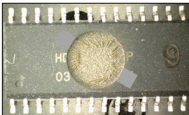
Fig. 42 Circular shape cavity decapsulated with laser for a final chemical etch.
