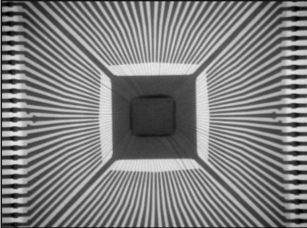
Fig. 33 Integrated circuit in QFP 100 and 0.5 mm pin pitch X-ray image.
