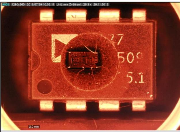
Fig. 60 OP177 component by AD package labeling illuminated with red radial lighting.
