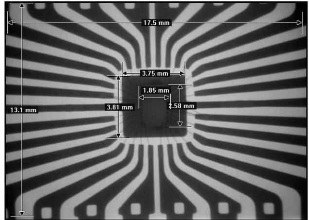
Fig. 30 EEPROM in DIL package X-ray image with dimensional values added.
