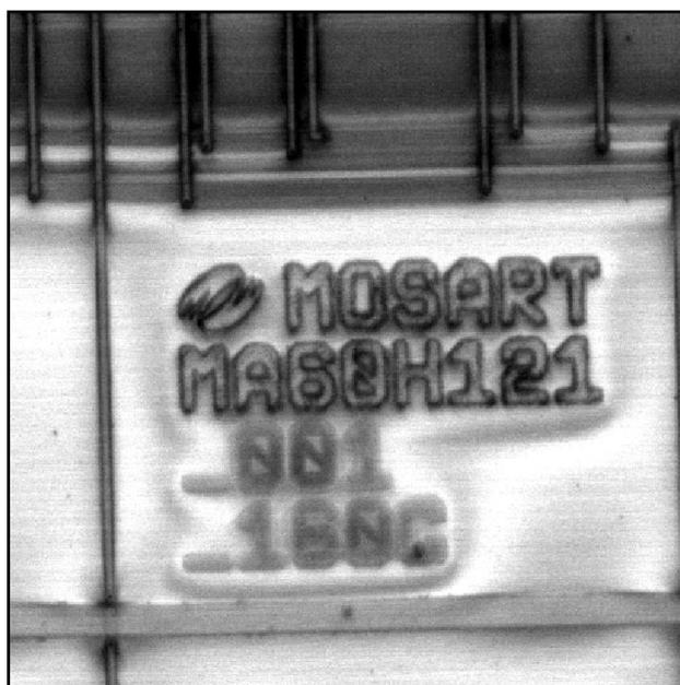
Fig. 47 Chip logo and chip marking view.
