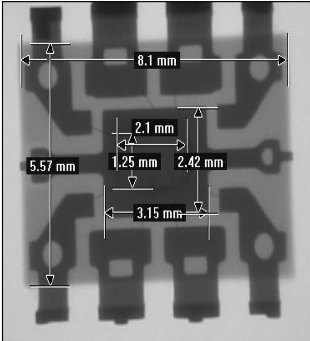
Fig. 28 Operational amplifier OP177 X-ray image with structural dimensions after scale calibration.
