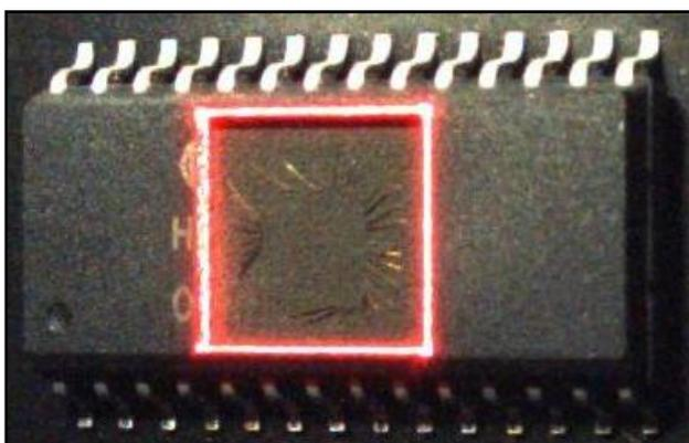
Fig. 39 Further package material ablated to reveal bonding gold wires.
