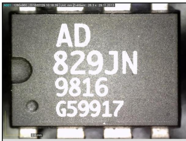
Fig. 22 Component package in a direct lighting.
