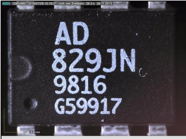
Fig. 23 Oblique lighting stressing surface and marking qualities.
