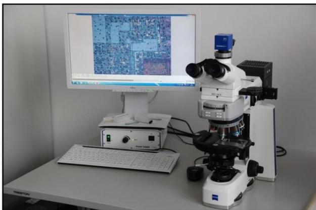
Fig. 18 Optical polarization microscope.
