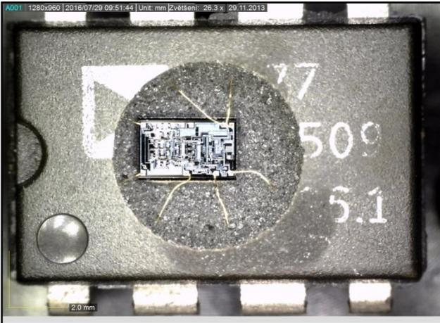
Fig.59 OP177 by Analog Devices package labeling illuminated with radial lighting.
