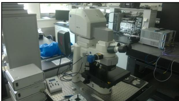
Fig. 19 Confocal microscope
