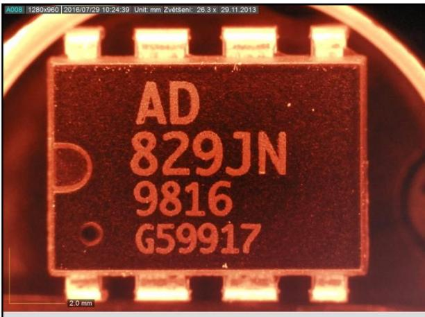
Fig. 24 Red or colour lighting can reveal some feature hidden in white lighting.
