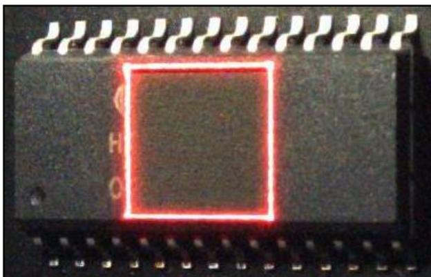
Fig. 38 Package material partially ablated with laser.
