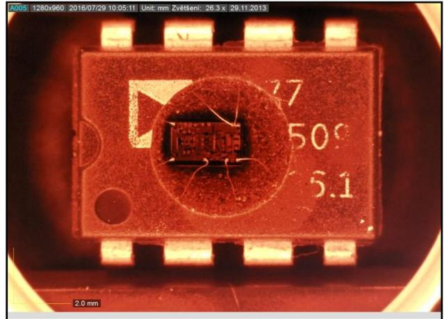
Fig. 62 OP177 by AD package labeling illuminated with red radial lighting combined with direct white vertical lighting.
