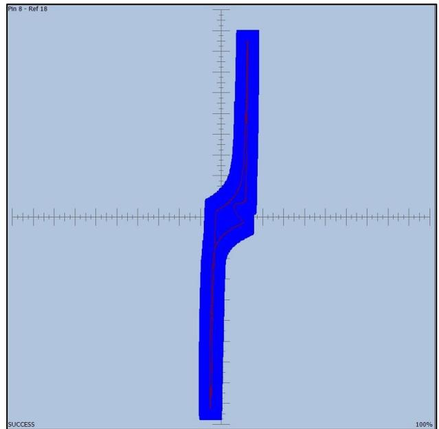
Fig. 10 High sensitivity mode pin print before laser ablation process started.
