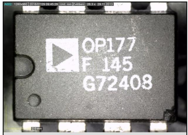
Fig.57 OP177 component by alleged AD package illuminated with direct vertical lighting.
