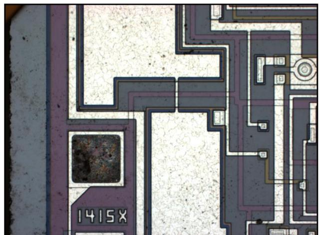
Fig. 64 Revealed PMI chip marking with polarization microscope magnification set to 200.
