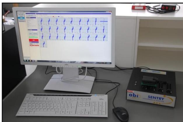
Fig. 15 ASA component pin print comparative evaluation workstation.
