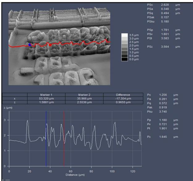
Fig. 50 The chip profile line with vertical differences.
