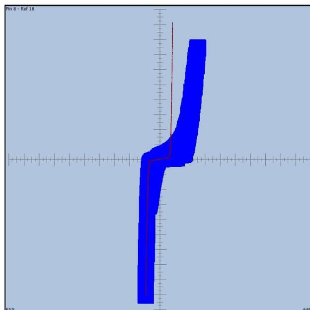
Fig. 13 High speed mode pin print affected by laser ablation process.
