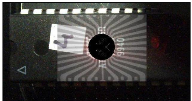
Fig. 37 X-ray picture combined with the laser camera picture.
