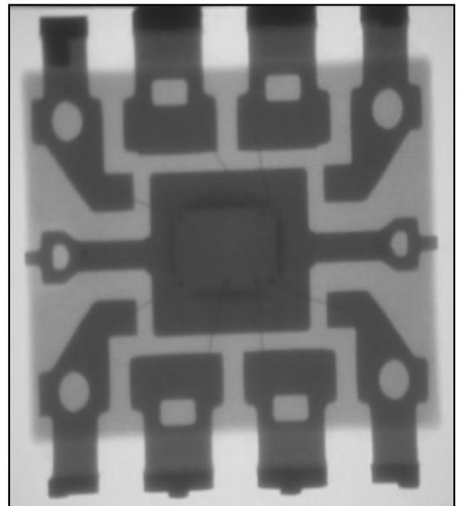
Fig. 27 Operational amplifier OP177 X-ray image.
