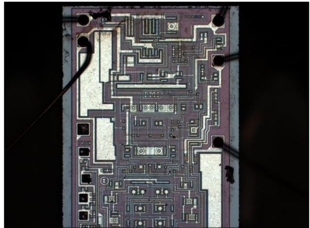
Fig. 63 The revealed PMI chip with polarization microscope magnification set to 50.
