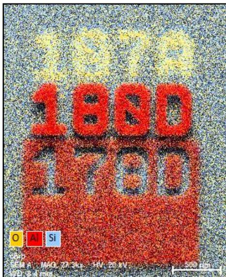
Fig. 56 Chip labeling material elements.
