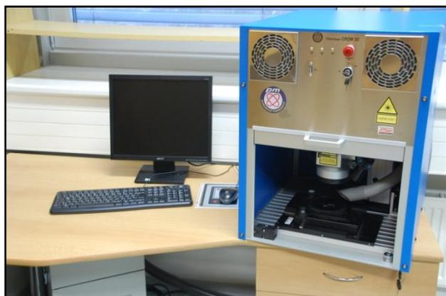
Fig.14 Fiber laser workstation with decapsulation and marking compartment open.
