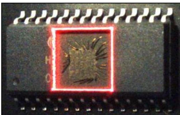
Fig. 40 Very thin protecting package material layer left.
