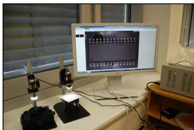
Fig. 17 Workstation for the first optical inspection of samples after laser ablation.
