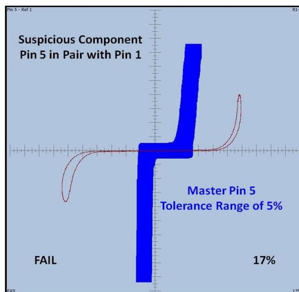
Fig.2 Pin 5 in pair with pin 1 I-V characteristics.
