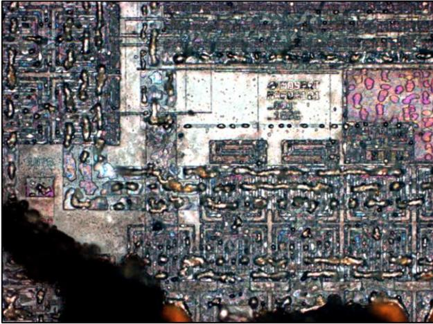
Fig. 7 Chip revealed only with fiber laser.
