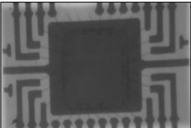
Fig. 35 MAX 211 in SOIC 28 package.
