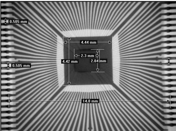
Fig. 34 Integrated circuit in QFP 100 and 0.5 mm pin pitch X-ray image with structural dimensions.
