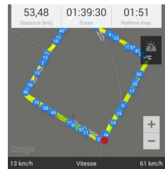
Fig 8: Smartphone solar cup circuit with measurement of speed & altitude every 1s. (4 right angle turns and 1 roundabout), measurement of distance & average speed plus an estimate of consumption, total altitude gain and vehicle performance.
