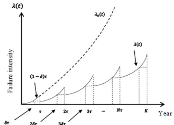
Fig 1. Failure intensity curve after Preventive Maintenance (PM). At  $i\tau, i=1,2,3,\dots,N$  the operator does a PM action.
