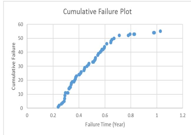
Fig. 2. Cumulative failure plot of bus. Plot looks convex which show that bus is deteriorating over time and follow NHPP process [6].
