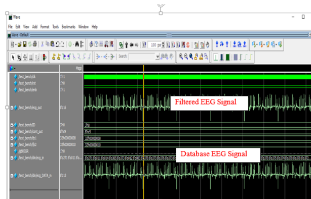
Fig.9. Artifacts removed simulated results of EEG signals for automatic detection of abnormality
