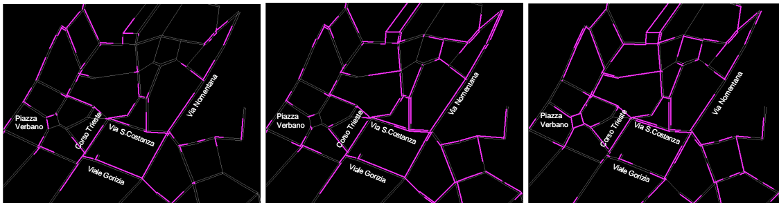
Fig. 11 Queue movement across the network as computed by Dynasmart in three different time instants.
