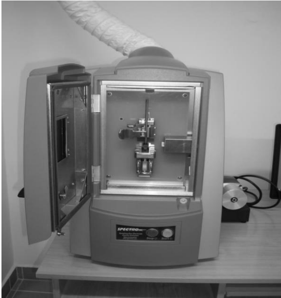
Fig. 7. General view of spectrometer Spectroil Q100
