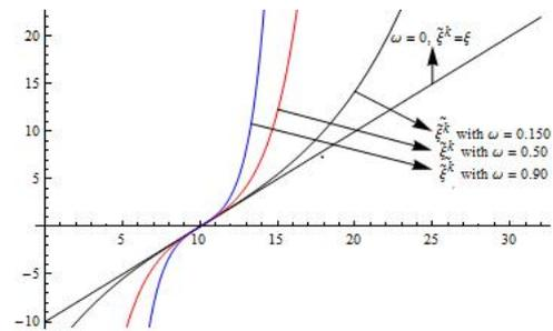
**Fig. 1.** A plot of (20)  $a=1, b=-10$ , with the parameter  $\omega$  assuming different values. The purpose and essence of this, is to demonstrate that as the parameter reduce to zero, the other curves converge to the straight line, where  $\tilde{\xi}^0 = \xi^0, \tilde{\xi}^1 = \xi^1, \tilde{\xi}^2 = \xi^2$ .
