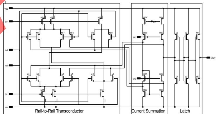
Fig.11.Rail-to-Rail comparator schematic
