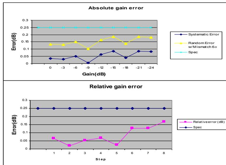
Fig.5. Absolute and Relative gain error of the PGA
