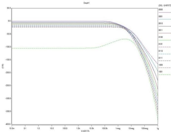
Fig.7. PGA frequency response
