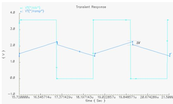
Fig.11: Ramp output before adjustment of Trim<3:3> (No continuity)
