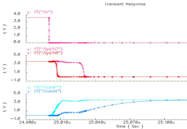
Fig.17. Turn-on Time and Dead-Time when PMOS goes off, and NMOS goes on
