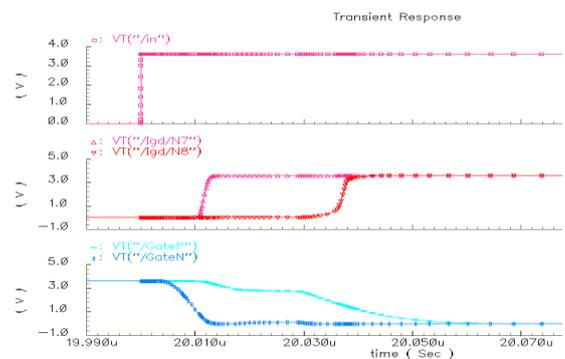
Fig.16. Turn-on Time and Dead-Time when NMOS goes off, and PMOS goes on
