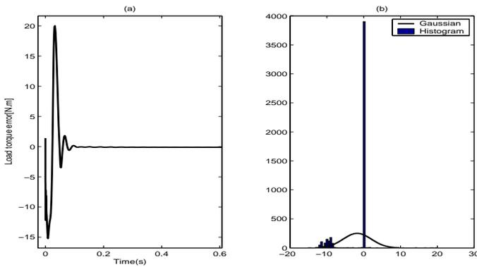
Figure 6: (a) Load torque error. (b) Gaussian and histogram of error load torque.
