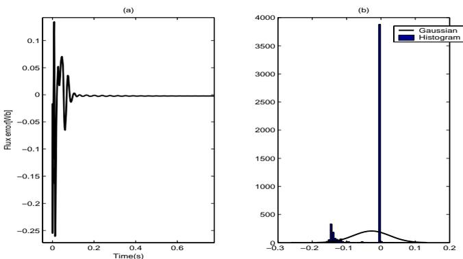
Figure 7: (a) Flux error. (b) Gaussian and histogram of error flux
