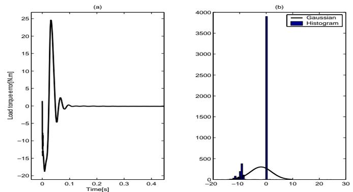
Figure 9: (a) Load torque error. (b) Gaussian and histogram of error load torque.
