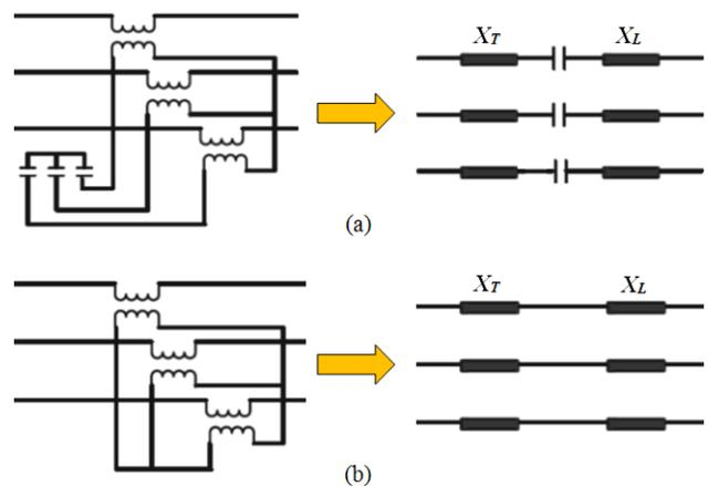
Fig. 2. Equivalent circuit of PWMSC.
