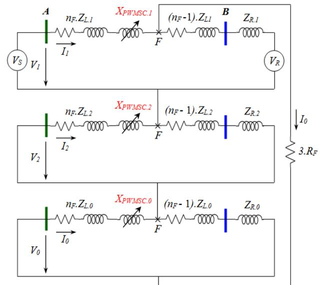
Fig. 4. Phase to ground fault equivalent circuit with PWMS device.
