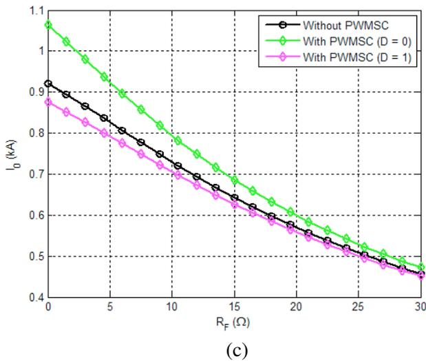
Fig. 7. Impact of fault resistance on current symmetrical components.
