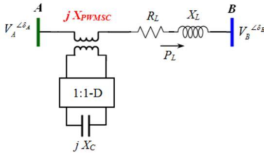
Fig. 3. Single distribution line diagram of PWMS.
