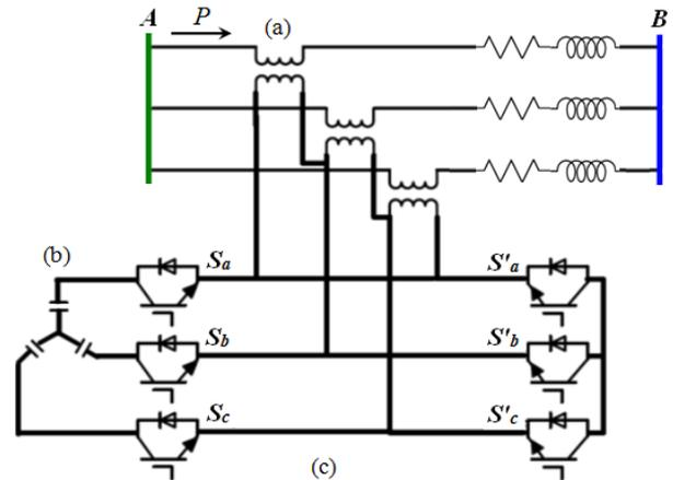
Fig. 1. Block diagram of PWMSC configuration [12-14].
