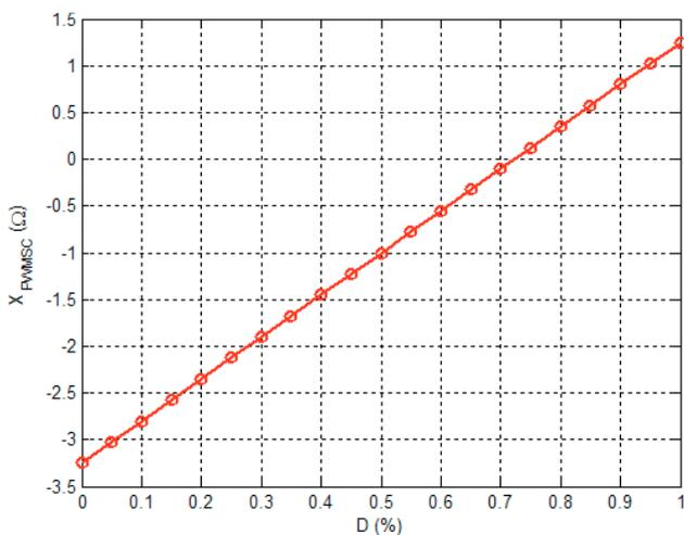
Fig. 6. Impact of duty cycle on the PWMSC apparent reactance.
