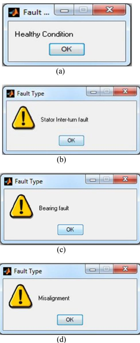
Fig.14 Testing result of the network in a message box (a) Healthy condition, (b) Stator Inter-turn fault condition, (c) Bearing fault condition, (d) Misalignment fault condition
